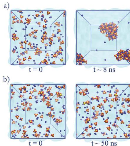
Fig. 4 Simulations of  $\text{Na}_2\text{SO}_4$ . (a) Original GAFF<sup>13,30–32</sup> parameters: aggregation becomes visible at 500 ps and large aggregates are seen at 8 ns. (b) Optimized anion–cation parameters: aggregation is not observed within the time scope of the simulation.
