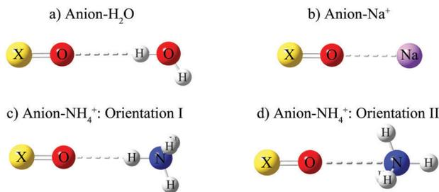
Fig. 2 Example configurations for the 1-D potential energy scans of anions: (a) with H<sub>2</sub>O, (b) with Na<sup>+</sup>, (c) with NH<sub>4</sub><sup>+</sup> in orientation I, (d) with NH<sub>4</sub><sup>+</sup> in orientation II. Orientation I results in a stronger hydrogen bond than orientation II.<sup>53</sup>
