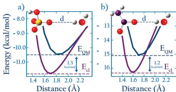
Fig. 7 (a)  $\text{HSO}_4^- \cdots \text{H}_2\text{O}$  (b)  $\text{CH}_3\text{COO}^- \cdots \text{H}_2\text{O}$ , 1D energy scan with both QM and classical methods. The curves in (a) are averaged over scans of different symmetries, as described in the ESI.†
