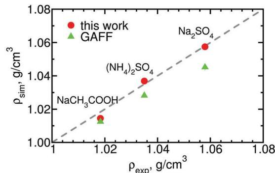
Fig. 8 Densities of three salts calculated using the optimized and the original GAFF parameters experimental densities.<sup>59</sup> The standard deviation of the simulation values is of order the height of the symbols. See ESI,† Table S6, for the numerical values.
