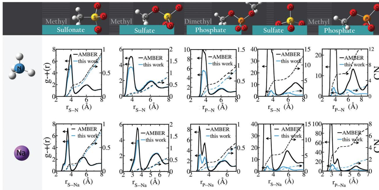
Fig. 6 Radial distribution functions of anion–cation pairs,  $g_{+-+}(r)$  (solid lines, left y-axes) and corresponding number integral (CN; dashed lines, right y-axes) using AMBER/GAFF parameters and using the optimized parameters.
