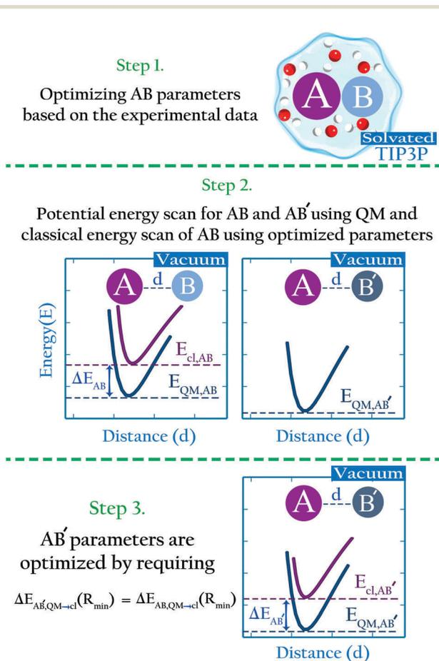
Fig. 1 The parameterization approach in this study.
