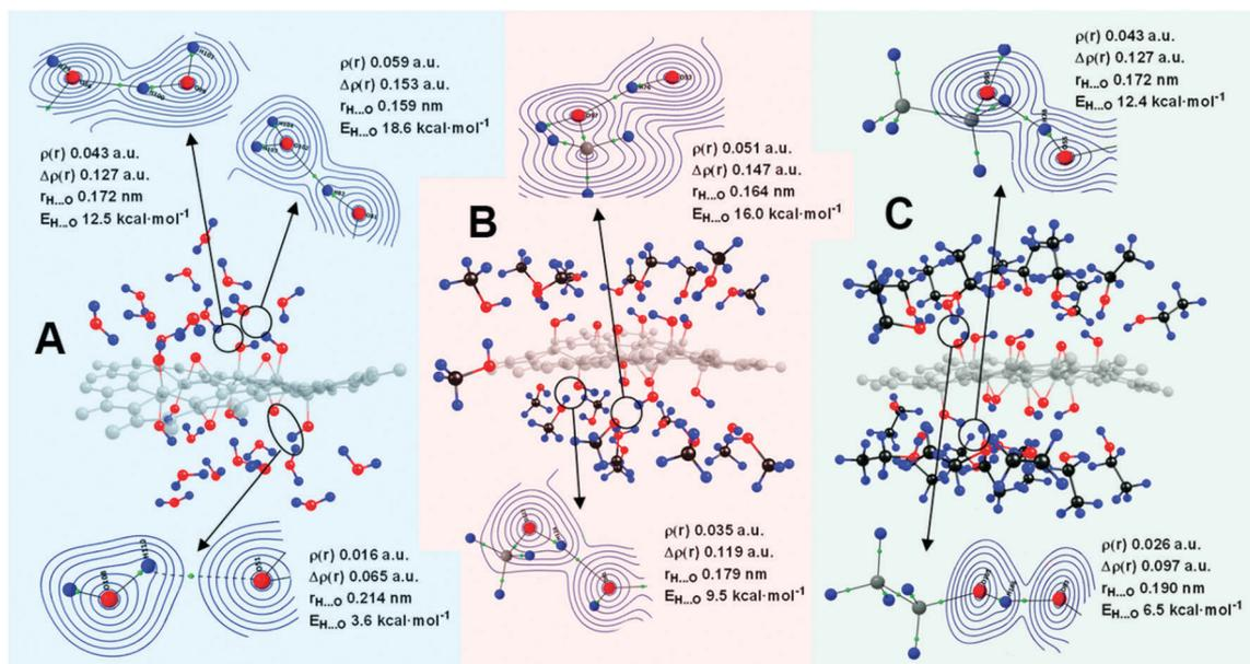
Fig. 1 Optimized structures of the solvates of graphene oxide with water (A), methanol (B) and ethanol (C). Hydrogen atoms are marked in blue, oxygen in red, carbon in black; BCPs are marked in green.
