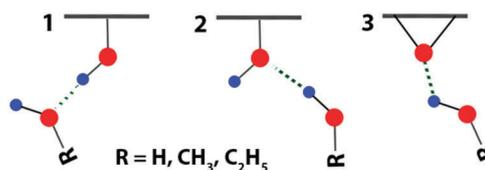
**Scheme 2** Schematic representation of the three different types of hydrogen bonding in the solvates of GO. Red balls denote the O atoms and blue balls the H atoms. (1) and (2) are the bonding to the tertiary alcohol. (3) is the bonding to the epoxide group.
