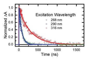
Fig. 6 Triplet state decay traces of 2-thiouracil at 0.6 mM in N<sub>2</sub>-saturated acetonitrile following excitation at 268, 290, or 316 nm. Each trace is an average across the triplet absorption band in the probe spectral range from ca. 630 to 710 nm.
