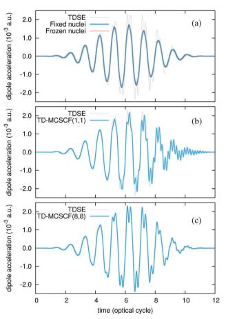
**Fig. 1** Time evolution of the dipole acceleration of one-dimensional  ${\rm H_2}^+$  exposed to a laser pulse with a wavelength of 800 nm and an intensity of  $1.0\times10^{14}$  W cm $^{-2}$ . Comparison of the results of fixed nuclei and frozen nuclei approximations (a), TD-MCSCF method with n=1 (b), and TD-MCSCF method with n=8 (c) with numerically exact TDSE results.
