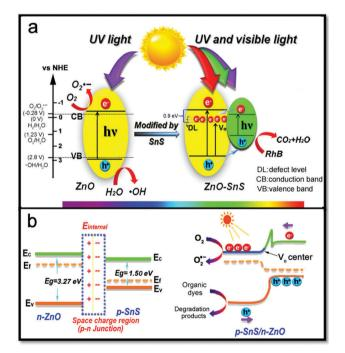
**Fig. 10** Mechanism for the degradation procedure of RhB with the 3D porous ZnO–SnS heterojunction as a catalyst: (a) the design of the p-n heterojunction with enhanced light harvesting range and (b) efficient carrier separation and transfer rate of the heterojunction.
