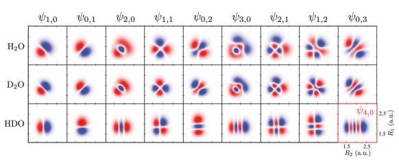
Fig. 11 Wave functions of the ground state of  $H_2O$ ,  $D_2O$  ( $\psi_{n_2,n_3}$ ) and HDO ( $\psi_{n_D,n_+}$ ). In the HDO,  $R_1$  represents the O-H bond and  $R_2$  the D-O bond. All wave functions are in the same scale.
