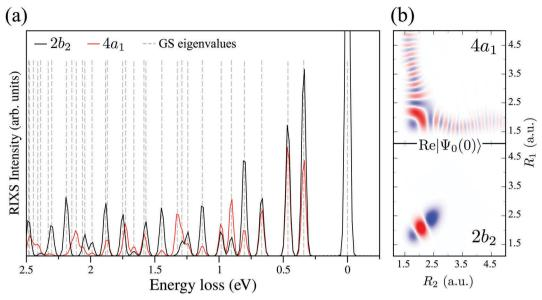
Fig. 13 (a) Theoretical HDO RIXS at the 4a<sub>1</sub> and 2b<sub>2</sub> resonances. The ground state eigenvalues are shown by the dashed lines and their assignment follows the energy order of Table 2. (b) Real part of the core-excited wave packet  $\Psi_0(0)$  at  $4a_1$  and  $2b_2$  resonances for HDO.
