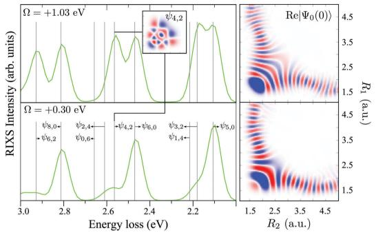
Fig. 10 Details of the RIXS at the  $4a_1$  resonance for different detuning values  $\Omega$ . The propensity rule, seen near the top of the XAS ( $\Omega = +0.30$  eV), is violated at large detuning ( $\Omega = +1.03$  eV) due to the change in the shape of the core-excited wave packet (right-hand side plots). The vertical lines show the energy position of the ground state wave functions.
