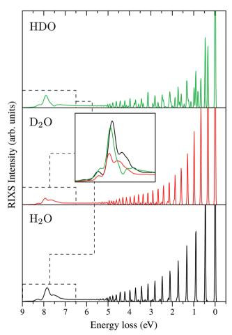
Fig. 14 RIXS spectra at the 4a<sub>1</sub> resonance for H<sub>2</sub>O, D<sub>2</sub>O and HDO, which show the formation of the "atomic" peak at around 7.5 eV. The detuning is the same as used in Fig. 12b. All spectra are given at the same intensity scale. The "atomic" peak exhibits a vibrational structure as it is formed by the emission transition from the core-excited fragment of dissociation \*OH.
