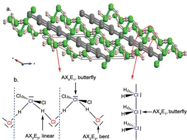
Fig. 8 (a) Crystal structure of *C2*- $\text{H}_4\text{Cl}_7$  at 350 GPa. The chlorine-based Kagomé layers are drawn in grey color. (b) VSEPR analyses of the zigzag HCl chain (left) and the linear chlorine one (right) in the *C2* phase.
