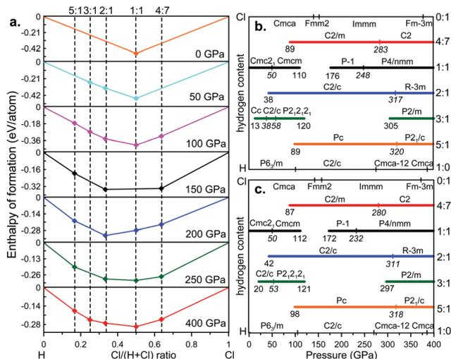
Fig. 1 (a) The calculated convex hulls of the H–Cl system at selected pressures. (b and c) Pressure–composition phase diagram of the H–Cl system between 0 and 400 GPa without (b) and with (c) ZPE corrections.
