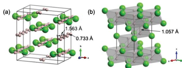
Fig. 4 Crystal structures of H<sub>2</sub>Cl in the (a) *C2/c* and (b)  $R\bar{3}m$  phases.
