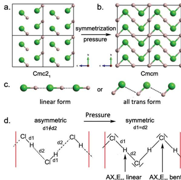
Fig. 2 (a and b) Crystal structures of *Cmc*2<sub>1</sub>- and *Cmcm*-HCl. The big green spheres represent Cl atoms, while the small pink ones denote H atoms. (c) 1D planar HCl chain in linear and all-trans forms. (d) Lewis structure for the 1D symmetrized zigzag chain with VSEPR AX<sub>n</sub>E<sub>m</sub> notation.
