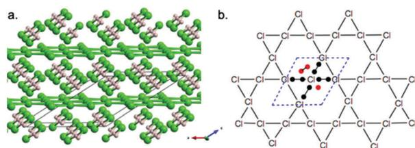
Fig. 7 (a) Crystal structure of *C2/m*- $\text{H}_4\text{Cl}_7$  at 100 GPa. (b) VSEPR analysis of the planar Kagomé  $(\text{Cl}_3)_2$  covalent layers.
