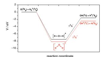
Fig. 1 Schematic representation of the potential energy profile along the minimum energy path for the ground ( $1^2A''$  PES) and first excited ( $1^2A'$  PES) potential energy surfaces.
