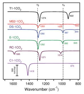
Fig. 11 Calculated (scaled) IRA spectra of  $CO_2$  adsorption on cluster models T1, MS2, DS, E, RC, and C1 with B3LYP. The experimental peaks are indicated by dashed lines for the lowest  $CO_2$  exposure. Frequencies and intensities tabulated in Table S26 (ESI†). All calculated spectra are Lorentzian broadened.
