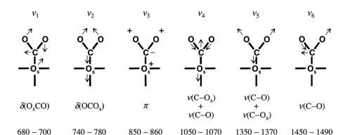
Fig. 5 Vibrational and bending modes in monodentate carbonate.  $O_s$  denotes the surface oxygen of the carbonate. The corresponding frequencies are labeled  $\nu_1$ – $\nu_6$ , from left to right. The bottom line shows the experimental frequencies assigned to the respective modes on the basis of conventional IR spectroscopy measurements on powdered samples. Figure modified from Fig. 5 of ref. 33.
