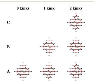
Fig. 10 Structures of three, four, and five adsorbed  $CO_2$  molecules on cluster T1 optimized with B3LYP from top views, simulating 0, 1, and 2 kinks in the chain of adsorbed carbonates, respectively. Color code: red, O; gray, Ca; cyan, C.
