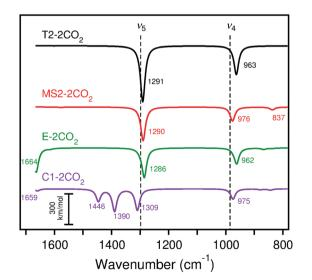
Fig. 12 Calculated (scaled) IRA spectra of CO2 adsorption on cluster models T2, MS2, E, and C1 with B3LYP. The experimental peaks are indicated by dashed lines for the lowest CO2 exposure. Frequencies and intensities tabulated in Table S27 (ESI†)
