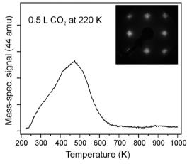
Fig. 6 Typical TPD spectrum of  $0.5 L CO_2$  exposed to CaO(001)/Mo(001) at 220 K. The inset shows the LEED pattern of the film with cross-like spots characteristic of mosaic structure. The heating rate is 3 K s<sup>-1</sup>.
