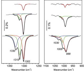
Fig. 4 Deconvoluted IRA spectra of CaO(001)/Mo(001) films exposed to  $\rm CO_2$  at increasing exposure from 0.1 L (top spectrum) to 1.1 L (bottom spectrum) at 110 K. The same color code is used as Fig. 3 for both panels.
