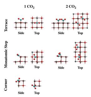
Fig. 8 Structures of adsorbed  $CO_2$  on terrace, monatomic step, and corner sites optimized with B3LYP from side (left) and top (right) views. The clusters have been truncated for clarity. Color code: red, O; gray, Ca; cyan, C.
