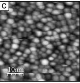
Fig. 1 Large-scale (a) and zoomed-in (b) STM images of a CaO(001) film grown on Mo(001). Points defects on terraces appear as depressions, and few are marked by circles. (c) STM image of a nanoparticulate CaO film prepared on Ru(0001). Tunneling conditions: bias 3.0 V, current 0.05 nA (a and b); 4.0 V, 0.05 nA (c).
