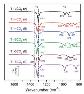
Fig. 13 Calculated (scaled) IRA spectra of adsorption of three to five CO<sub>2</sub> molecules on cluster model T1 with B3LYP. The experimental peaks are indicated by dashed lines. The experimental  $\nu_5$  mode corresponds to the highest and lowest observed peaks from spectral deconvolution.
