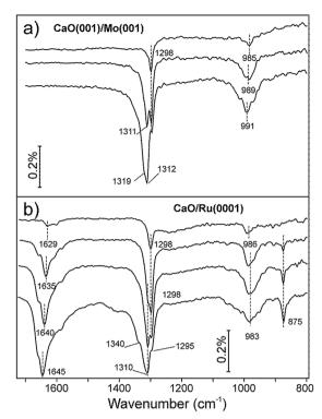
Fig. 2 IRA spectra of (a) CaO(001)/Mo(001) and (b) CaO/Ru(0001) films exposed to  $CO_2$  at increasing exposure from 0.1 L (top spectrum) to 1.1 L (bottom spectrum) at 300 K. The spectra are offset for clarity.
