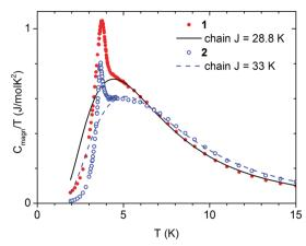
Fig. 7 Magnetic contribution  $C_{\text{magn}}$  of the specific heat, obtained for compounds **1** and **2**, shown as C/T. The lines denote the fitted contribution related to the exchange interaction J within chains of Ising spins.
