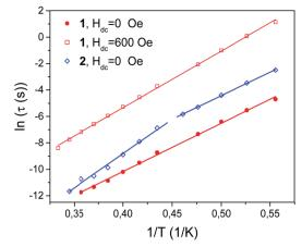
Fig. 10 Temperature dependence of the relaxation time  $\tau$  determined at  $H_{\rm dc}=0$  Oe for 1 and 2 and at  $H_{\rm dc}=600$  Oe for 1. Straight lines were fitted using the Arrhenius equation.
