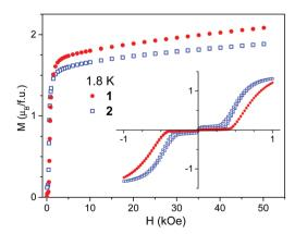
**Fig. 5** Field dependent magnetization measured at 1.8 K for compounds **1** and **2**. Inset shows magnetic hysteresis loops registered in the low field range.
