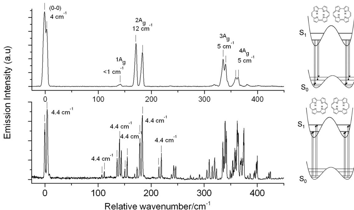
Fig. 2 Spectra of porphycene isolated in a supersonic jet. Bottom, fluorescence excitation (LIF) and top, fluorescence recorded for excitation into the 0–0 origin band ( $16\,163\text{ cm}^{-1}$ ). Tunnelling splitting values are presented for selected vibronic levels. Frequencies are given relative to the 0–0 excitation energy.
