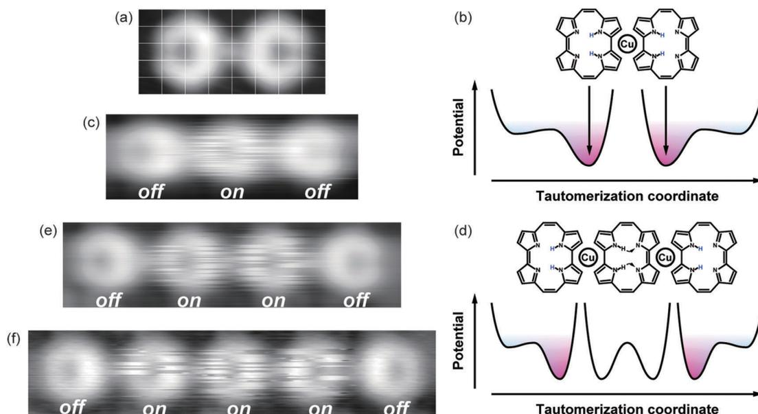
**Fig. 9** One-dimensional porphycene assemblies on a Cu(110) surface at 5 K. (a) Dimer. (b) Schematic of the dimer and the tautomerization potential. (c) Trimer. (d) Schematic of the trimer and the tautomerization potential. (e) Tetramer. (f) Pentamer. All STM images were obtained at  $V_{\text{bias}}$  of 300 mV which is sufficiently higher than the threshold required to induce the *cis*  $\leftrightarrow$  *cis* tautomerization.
