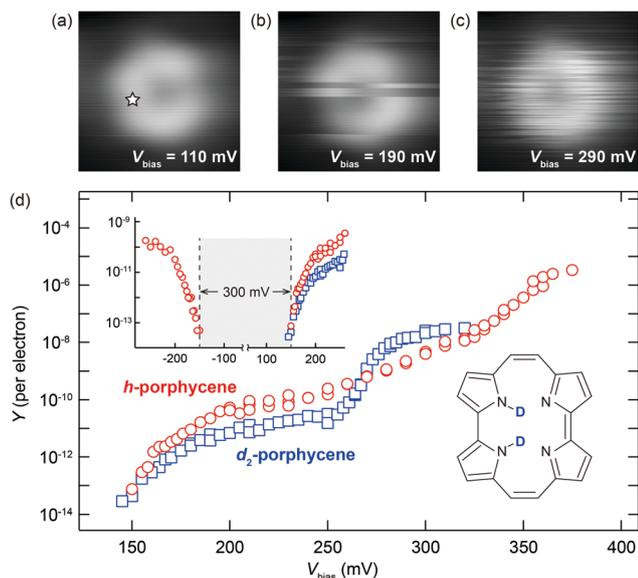
**Fig. 8** Electron-induced *cis*  $\leftrightarrow$  *cis* tautomerization of porphycene on a Cu(110) surface. (a–c), STM images at 5 K obtained at different bias voltages. (d) Bias voltage dependence of the tautomerization yield (STM action spectra) measured for *h*- and *d*<sub>2</sub>-porphycene. The inset displays the yields at both bias polarities in the regime of the threshold voltage.
