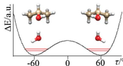
Fig. 3 The tunneling motion in of IP–W–GAI is predominantly due to the internal rotation of the hydroxyl group, accompanied by a structural relaxation of the "free" water hydrogen.
