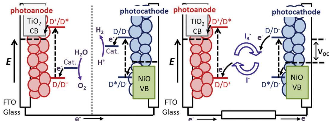
Fig. 1 Schematic energy level diagram of a photoelectrosynthesis cell for splitting H<sub>2</sub>O (left) and a tandem DSC where a n-type photoanode and a p-type photocathode are incorporated into one device (right).
