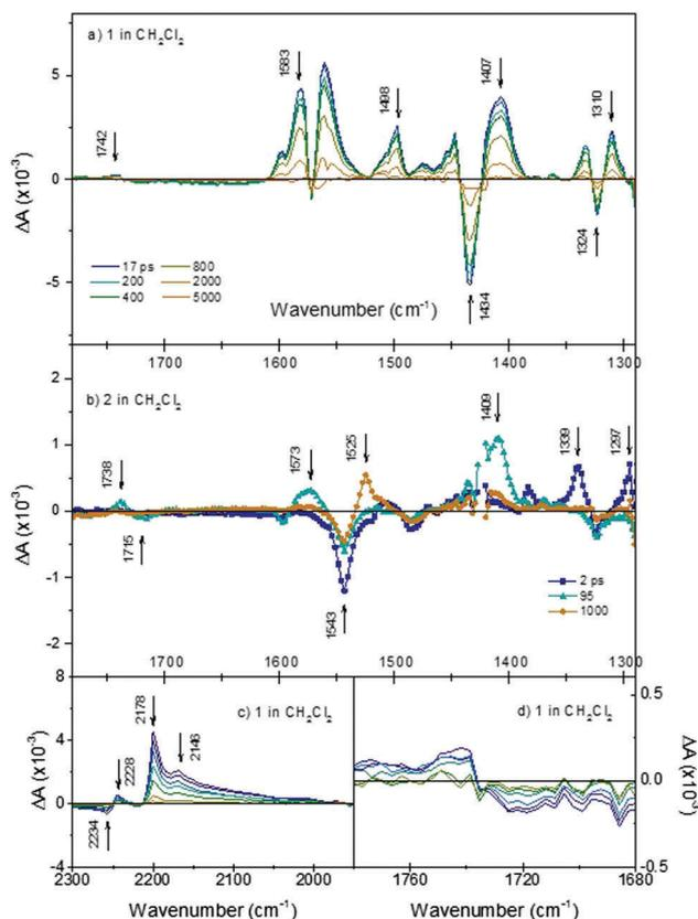
Fig. 4 TRIR spectra after excitation at 532 nm of (a) **1** in  $\text{CH}_2\text{Cl}_2$  across the fingerprint regions at various time delays; (b) **2** in  $\text{CH}_2\text{Cl}_2$  fingerprint region at 2 ps (blue line and squares); 95 ps (cyan line and triangles) and 100 ps (orange line and circles); (c) **1** in  $\text{CH}_2\text{Cl}_2$  in the  $\nu(\text{C}\equiv\text{N})$  region; (d) **1** in  $\text{CH}_2\text{Cl}_2$  in the  $\nu(\text{C}=\text{O})$  region.
