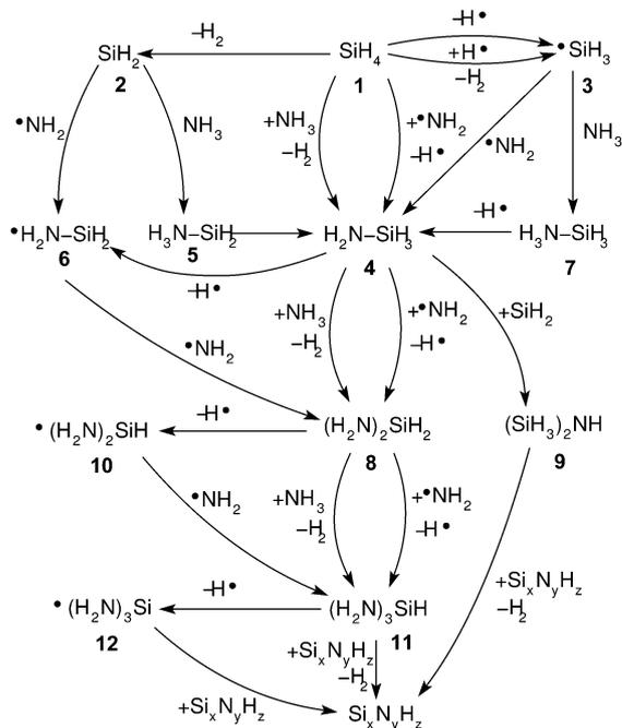
Fig. 1 Possible reactions in plasma created from a gas mixture of ammonia and silane. Si<sub>x</sub>N<sub>y</sub>H<sub>z</sub> represents a surface of the silicon nitride.
