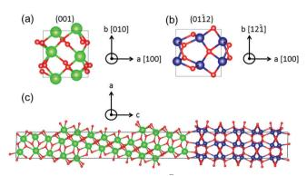
Fig. 2 (a) m-ZrO<sub>2</sub>(001) and (b)  $Cr_2O_3(01\overline{1}2)$  surface cross sections and (c) relaxed interface. Oxygen ions are drawn small and red, Cr ions are medium-sized and blue, Zr ions are largest and green. This figure is generated with visualization software VESTA.56
