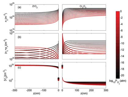
Fig. 8 Spatially-resolved concentrations of (a) electrons, (b) sum of electrons and holes and (c) V<sub>0</sub><sup>•</sup> as a function of oxygen partial pressure at T = 1200 K. Circles and squares in panel (c) represent the concentrations in the core layer on the ZrO2 and Cr2O3 sides, respectively
