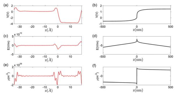
Fig. 9 Macroscopic average of (a) electrostatic potential  $V_r$  (c) electric field E and (e) charge density  $\rho$  from the perfect interface calculated by DFT at 0 K, compared with the same quantities (b), (d) and (f) contributed by the redistribution of defects at T = 1200 K and  $P_{O_2} = 10^{-5}$  atm.
