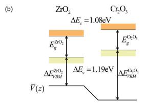
Fig. 3 (a) Planar (solid black line) and macroscopic average (dashed red line) of electrostatic potential across the ZrO<sub>2</sub>/Cr<sub>2</sub>O<sub>3</sub> interface obtained from DFT calculation.  $\Delta \bar{V}^{ZrO_2-Cr_2O_3} = 3.77 \text{ V}$  is the potential difference on both sides of the interface where flat potentials are reached. (b) Aligned band positions. Band gaps of ZrO2 and Cr2O3 from DFT calculations are 3.49 eV and 3.38 eV, respectively.
