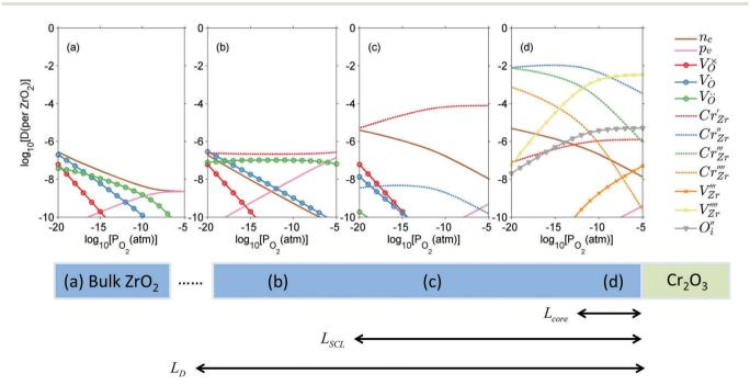
Fig. 6 Defect concentrations at 1200 K and different oxygen partial pressures in  $ZrO_2$  (a) in bulk, (b) far from the space-charge zone but within the reach of Cr defects, (c) outside the core layer within the space-charge zone, and (d) in the core layer.
