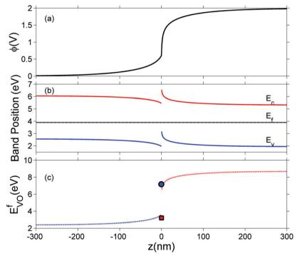
Fig. 4 (a) Electrostatic potential, (b) band edges positions for valence band  $E_v$  and conduction band  $E_c$ , and the Fermi level  $E_t$ , (c) formation energy of doubly charged oxygen vacancy calculated at 1200 K and  $P_{O_2} = 10^{-5}$  atm. The interface is placed at z = 0 with  $ZrO_2$  on the left side and  $Cr_2O_3$  on the right side. In (c), the blue circle ( $ZrO_2$  side) and red square ( $Cr_2O_3$  side) show explicitly the formation energy in core layers on each side.
