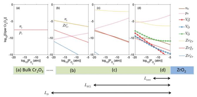
Fig. 7 Defect concentrations in  $Cr_2O_3$  at 1200 K and different oxygen partial pressures (a) in bulk, (b) far from the space-charge zone but within the reach of Zr defects, (c) outside the core layer within the space-charge zone, and (d) in the core layer.
