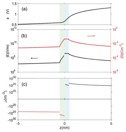
Fig. 5 (a) Electrostatic potential  $\phi$ , (b) the magnitude of the electric field E and electric displacement field D and (c) charge concentration  $\rho$  close to the interface. Regions with green and blue background color represent core layer on  $ZrO_2$  and  $Cr_2O_3$  side, respectively.
