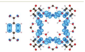
Fig. 2 Highest occupied states (HOCO) are localized on the aromatic organic group, while the lowest unoccupied states (LUCO) are localized on the octameric TiO<sub>2</sub> units for NH<sub>2</sub>-MIL-125(Ti).<sup>61</sup> Reproduced with permission from Wiley.
