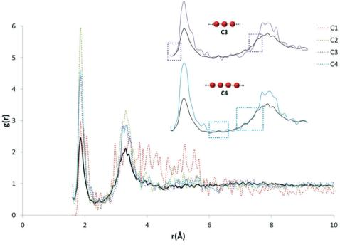
Fig. 5 An example of the initial overlay analysis of motif RDFs with the original HW···OW RDF. Discrete features for both the C3 (purple) and C4 motif (blue) appear to be present in the original function. Other discrete chain motifs are also represented here, as indicated by the legend (top right).
