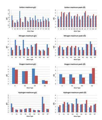
**Fig. 6** The maximum peak (defined by g(r)) for each RDF pair profile (each atom type with HW and OW) was determined. These bar graphs show the q(r) value for the maximum peak of each atom type with OW (blue bars) and HW (red bars) on the left, with the distance at which these peaks were found plotted on the bar graphs on the right.
