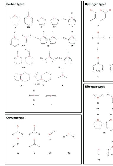
Fig. 1 Schematic representations of AMBER atom types. The red colour represents the atom being typed. The code below each schematic refers to the code assigned by the AMBER routine. R groups represent any atom, and X groups represent either N or O. Dotted lines represent undefined bond order, and solid lines represent conventional nomenclature of bonds.
