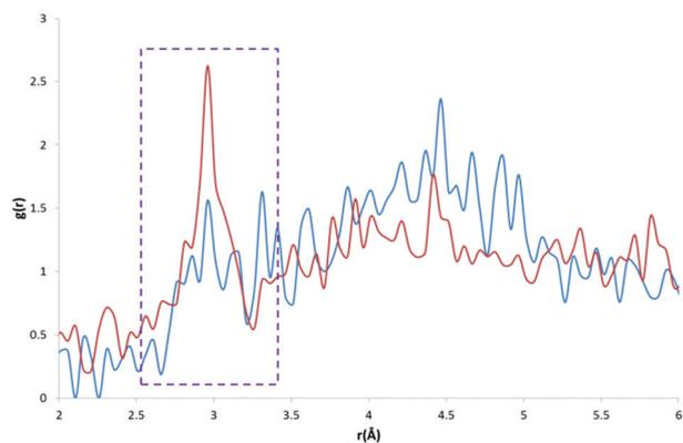
Fig. 8 CC $\cdots$ HW RDF (blue) and CK $\cdots$ HW RDF (red) with a much larger peak apparent at  $\sim 3$  Å in the CK $\cdots$ HW profile (outlined in purple).
