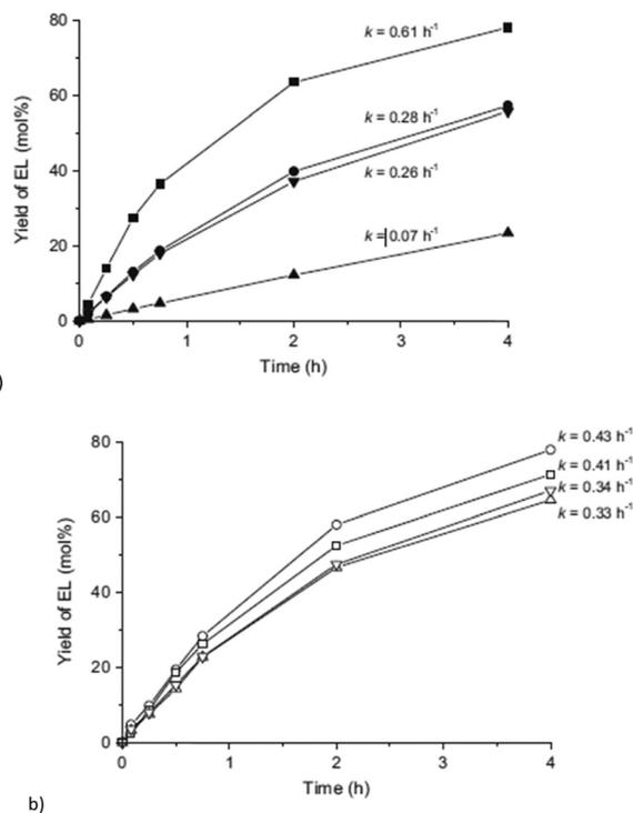
**Fig. 29** Yield of ethyl levulinate (EL) obtained over (a) UiO-66, batches B1 to B4 (from top to bottom), (b) UiO-66-NH<sub>2</sub>, batches A1 to A4 (from top to bottom). For each curve, the calculated pseudo-first-order kinetic rate constant is indicated. Reprinted from ref. 155. Copyright 2015 with permission from Elsevier.
