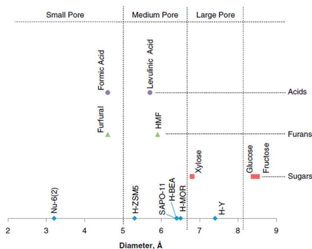
**Fig. 7** Comparison of catalyst pore dimensions (blue dots) and molecular dimensions of carbohydrates (red) and biomass-derived platform chemicals (green and violet). Reprinted from ref. 13. Copyright 2012 with permission from Elsevier.
