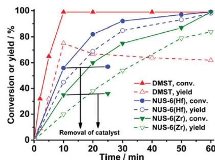
**Fig. 20** Kinetic study of fructose dehydration to 5-HMF with NUS-6 and DMST catalysts (DMST = dimethyl-2-sulfoterephthalate). Conditions: fructose (50 mg), 3.5 mol% catalyst (2.7 mg for DMST, 35 mg for NUS-6(Zr), 50 mg for NUS-6(Hf)), DMSO (1 mL), 100 °C, 1 h. Reprinted with permission from ref. 124. Copyright 2016, American Chemical Society.
