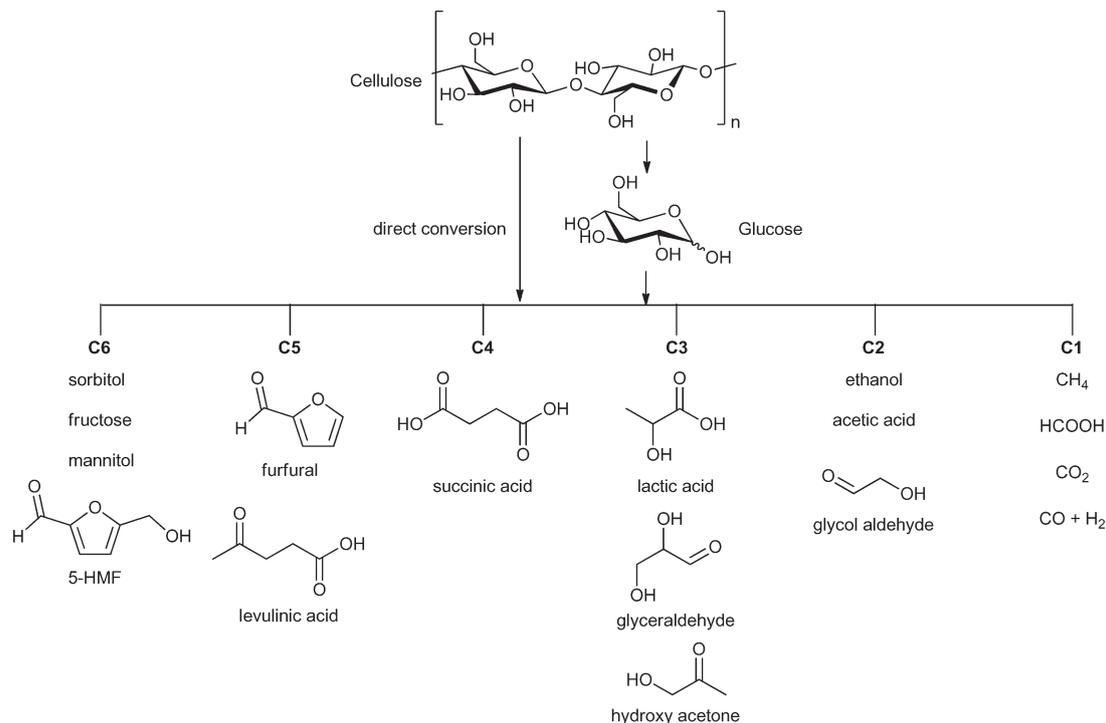
Fig. 2 Possible valuable chemicals based on carbohydrate feedstock. Figure modified from ref. 15.
