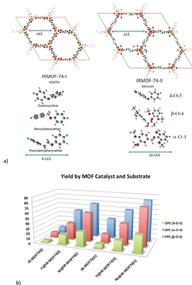
**Fig. 33** (a) Pore diameters of IRMOF-74(I) and IRMOF-74(II) and largest intramolecular distances in the aromatic ether compounds, corresponding to a straight line between the blue-highlighted atoms in the optimized geometries. (b) Conversion efficiencies of the substrates into the corresponding hydrocarbon and phenol at 120 °C under 10 bar hydrogen. Reprinted with permission from ref. 166. Copyright 2016, American Chemical Society.
