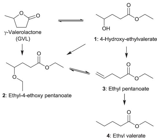
Fig. 27 Reaction pathways of GVL conversion in ethanol; obtainable products 1–4 with MIL-101Cr-SO<sub>3</sub>H or Pd@MIL-101Cr-SO<sub>3</sub>H are depicted. Additional by-products were omitted for clarity. Modified from ref. 153.
