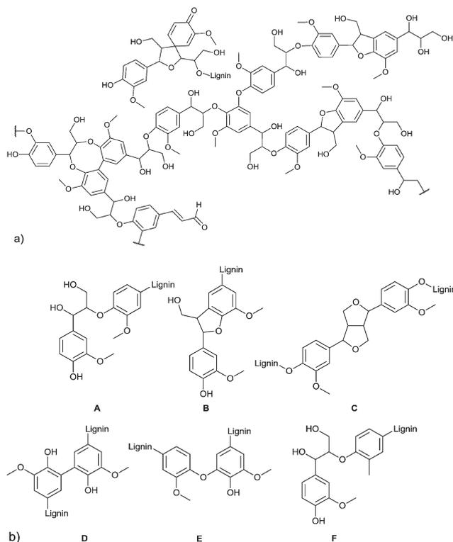
**Fig. 4** (a) Structural motifs of softwood lignin. (b) Six common linkages found in lignin: A =  $\beta$ -O-4, B =  $\beta$ -5, C =  $\beta$ - $\beta'$ , D = 5-5', E = 4-O-5, F =  $\beta$ -1'. Figures redrawn from ref. 19.
