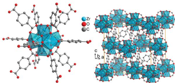
Fig. 9 Structure of zirconium terephthalate UiO-66Zr. The SBU is a hexanuclear and octahedral cluster of six edge-sharing  $\text{ZrO}_8$  square antiprisms, which is connected to 12 neighboring SBUs in a face-centered cubic (fcc) packing arrangement. The structure was drawn from deposited cif-files under CCDC 837796 (UiO-66).<sup>81</sup>
