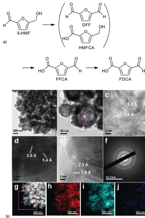
**Fig. 26** (a) Products of HMF oxidation. (b) (a–e) HRTEM images of FeCo/C(500); (f) SAED pattern; (g) HAADF-STEM images of FeCo/C(500) and the corresponding elemental mappings of (h) Fe, (i) Co and (j) C. Redrawn and reprinted from ref. 149. Copyright 2016, with permission from the Royal Society of Chemistry.
