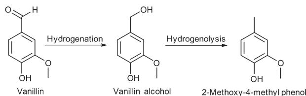
**Scheme 12** Hydrodeoxygenation of vanillin to 2-methoxy-4-methyl phenol.
