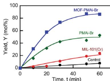
Fig. 17 5-HMF yield (%) from fructose at 100 °C. Conditions: DMSO, 5 mL; D-fructose concentration (C<sub>fo</sub>), 0.555 mol L<sup>-1</sup>; catalyst loading, 50 mg mL<sup>-1</sup>. Control: DMSO solvent with no catalysts added. Reprinted with permission from ref. 122. Copyright 2014, American Chemical Society.
