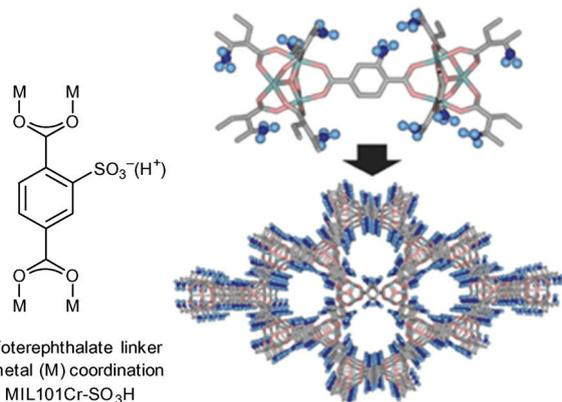
**Fig. 12** 2-Sulfoterephthalate, MIL-101Cr-SO<sub>3</sub>H SBU and network. Adapted from ref. 34. Copyright 2011 with permission from John Wiley and Sons.
