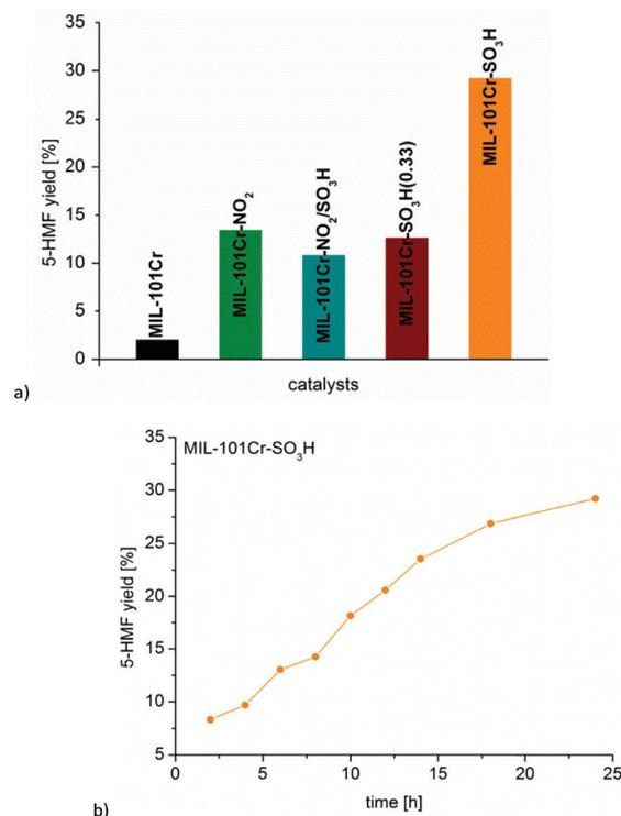
**Fig. 21** (a) 5-HMF yield from glucose with different MIL-101Cr catalysts. (b) Time-dependent conversion for MIL-101Cr-SO<sub>3</sub>H (glucose 223 mg, 1.24 mmol, catalyst 5.22 × 10<sup>-5</sup> mol, 5 mL THF/H<sub>2</sub>O v: v 39:1, 130 °C, 24 h). Reprinted from ref. 134. Copyright 2016 with permission from the Royal Society of Chemistry.
