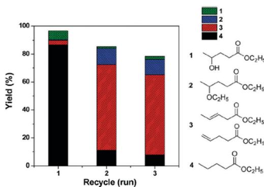
Fig. 28 Reusability and product distribution of Pd@MIL-101-SO<sub>3</sub>H(80) catalyst in GVL ring opening reactions. Reaction conditions: 10 mmol of GVL, 5820 mL of ethanol, 250 °C, 10 h, 3 MPa H<sub>2</sub>. Reprinted from ref. 153. Copyright 2014 with permission from the Royal Society of Chemistry.
