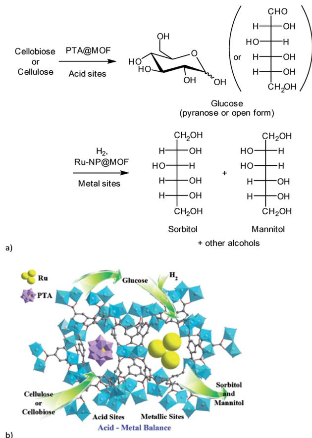
**Fig. 14** (a) Reaction scheme of cellulose conversion to sorbitol with Ru(nanoparticle)/PTA@MIL-100Cr; (b) proposed function of MOF composite catalyst. Redrawn and reprinted from ref. 112. Copyright 2013 with permission from John Wiley and Sons.
