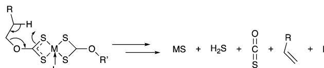
Scheme 1 A generalised breakdown mechanism proposal for the xanthate precursors. M = Ca, Ba or Cu, L = i PrOH or PPh 3 , R = i Pr or 2-methoxyethyl.
