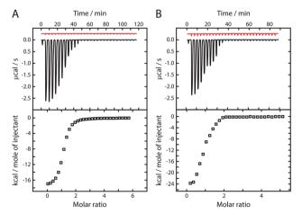
Fig. 1 Representative ITC thermograms (upper panels) and isotherm plots (lower panels), showing consecutive injections of (A) apo mACPa against mKRa and (B) apo mACPb against mKRb, in the presence of excess NADPH. Thermogram traces for dilution control experiments are displayed in the upper panels in red.
