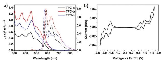
Fig. 2 (a) UV-vis spectra (solid) and photoluminescence (PL) spectra (dashed, excited at 455 nm) of TPCa–c ( $1.0 \times 10^{-6} \text{ M}$  in toluene); and (b) cyclic voltammograms of TPCb in DCM (0.5 mM) containing 0.1 M Bu<sub>4</sub>NPF<sub>6</sub>. Potentials are reported vs. the Fc/Fc<sup>+</sup> redox couple as a standard, scan rate = 50 mV s<sup>-1</sup>.
