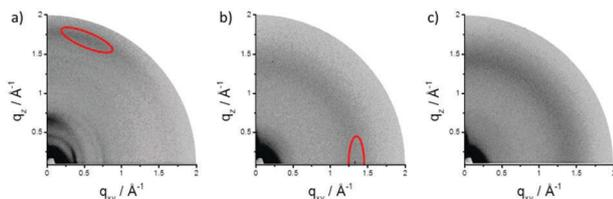
Fig. 4 GIWAXS patterns for thin films of (a) TPCa, (b) TPCb and (c) TPCc. Reflections corresponding to molecular stacking are indicated in red.
