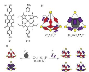
Fig. 12 (a) Diamine sub-components S1 and S17, based on either a NDI or porphyrin backbone; (b) the corresponding tetrahedral cages showing the distinct host-guest chemistry of each cage; (c) a dynamic library which rearranges according to the type of stimulus introduced.
