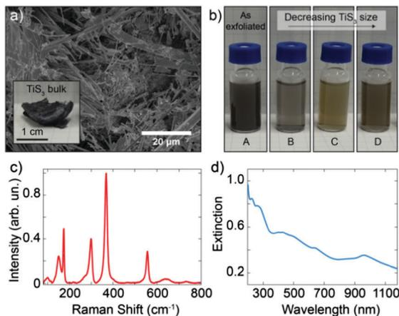
**Fig. 1** (a) SEM image of the lamellar  $\text{TiS}_3$  bulk material. Inset: Photograph of bulk  $\text{TiS}_3$ . (b) Optical image of the colloidal suspensions of exfoliated  $\text{TiS}_3$  in IPA. (c) Raman spectrum (normalized at  $368\text{ cm}^{-1}$ ) and (d) UV-Vis-NIR spectrum of colloidal suspension D.
