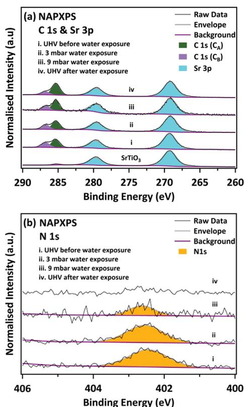
Fig. 2 NAPXPS spectra of (a) C 1s & Sr 3p, and (b) N 1s core levels before/during/after water exposure. All spectra are normalised to the corresponding integrated area of the Sr 3d<sub>5/2</sub> peak.
