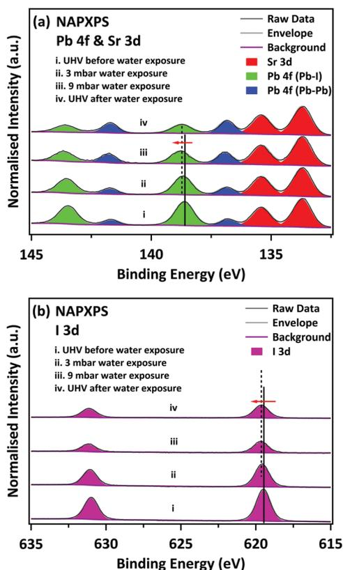
**Fig. 1** NAPXPS spectra of (a) Pb 4f & Sr 3d, and (b) I 3d core levels under various conditions as noted (before/during/after water exposure). All the spectra are normalised to the corresponding integrated area of the Sr  $3d_{5/2}$  peak.
