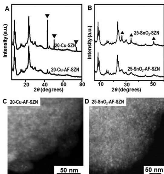
Fig. 2 (A and B) XRD patterns (bottom) and (C and D) STEM images of 20 wt% Cu and 25 wt% SnO<sub>2</sub> supported AF-SZN samples. (A and B) XRD patterns (top) of 20 wt% Cu and 25 wt% SnO<sub>2</sub> supported SZN samples are also displayed for comparison. The XRD peaks of metallic Cu and SnO<sub>2</sub> are marked with an inverted triangle and a triangle.
