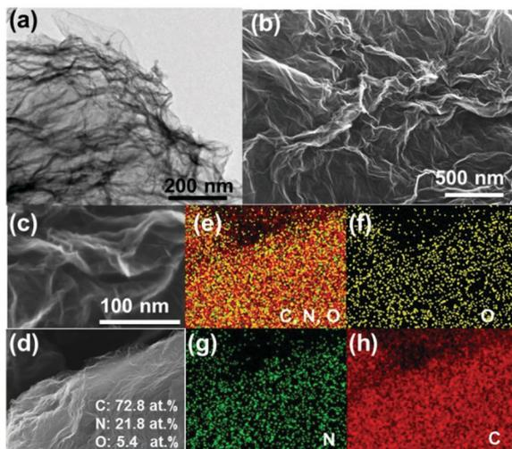
Fig. 1 (a) TEM, (b–d) SEM and (e–h) elemental mapping images for N-doped graphene nanosheets.
