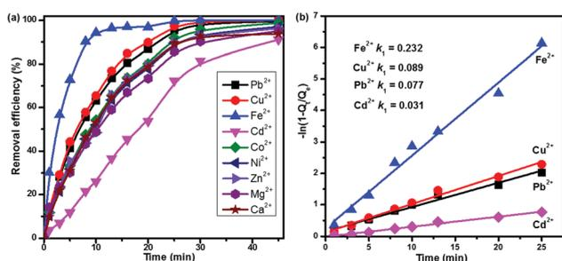
Fig. 3 MCDI performance for multiple ions removal: (a) time-dependent efficiency and (b) kinetics for  $\text{Fe}^{2+}$ ,  $\text{Cu}^{2+}$ ,  $\text{Pb}^{2+}$ , and  $\text{Cd}^{2+}$  ( $\sim 10$  ppm for each metal ion, flow rate:  $50 \text{ ml min}^{-1}$ , 25 mg materials, 100 ml solution, 1.2 V).
