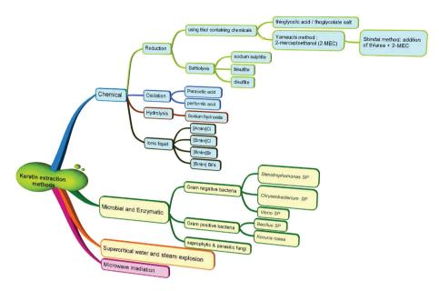
Fig. 2 Classification of various methods used for the extraction of keratin from keratin-rich materials, such as wool, feathers and hooves.
