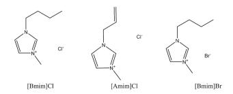
Fig. 5 Schematic structures of three major ionic liquids that have been widely used for the dissolution of keratin fibres. 1-Butvl-3-methylimidazolium chloride [Bmim]Cl, 1-allyl-3-methylimidazolium chloride [Amim]Cl, and 1-butyl-3-methylimidazolium bromide [Bmim]Br.
