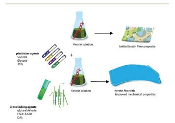
Fig. 10 Effect of different plasticizers and crosslinking agents on the mechanical properties of the keratin film.
