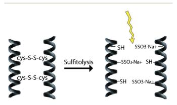
Fig. 4 Schematic diagram of the sulfitolysis reaction that breaks the strong disulfide bonds of the keratin fibre.
