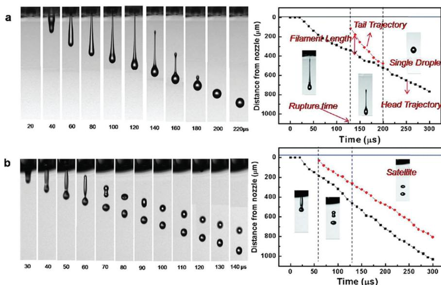
**Fig. 3** (Left) Representative photo sequence of droplet formation and (right) representative trajectories of the ejected droplets as a function of the elapsed time for bio-inks with varying values of  $Z$ : (a)  $Z = 2.17$ ; (b)  $Z = 17.32$ . "Reprinted (adapted) with permission from ref. 45. Copyright (2009) American Chemical Society".
