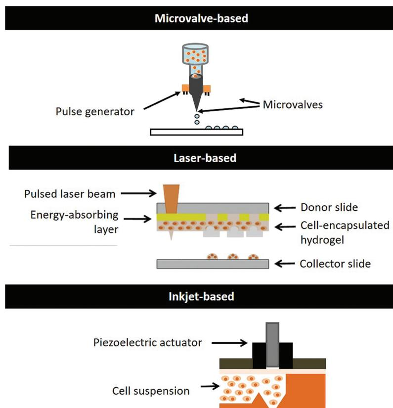
Fig. 1 Schematic drawing of different DOD bioprinting systems.
