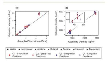
Fig. 4 Comparison between the accepted and calculated viscosities (a) and densities (b) of the probed fluids. The values of  $\eta$  and  $\rho$  derived from the measurements compare well with the accepted values, as evidenced by their collapse onto the line of unity gradient. The inset in (b) highlights the data points at lower densities.
