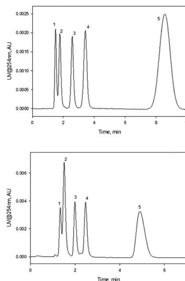
**Fig. 4** Selectivity of UiO-66@SiO<sub>2</sub> stationary phases towards positional isomers. Mobile phase – 0.2 ml min<sup>-1</sup> of *n*-hexane, 25 °C, 2  $\mu$ L injections of analytes (50  $\mu$ g mL<sup>-1</sup>) in mobile phase, UV detection at 254 nm. Analytes: 1 – propyl benzene, 2 – cumene, 3 – *p*-xylene, 4 – *m*-xylene, 5 – *o*-xylene. Columns: UiO-66(2x)@SiO<sub>2</sub>(5) (top) and UiO-66(1x)@SiO<sub>2</sub>(5) (bottom).
