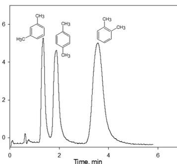
**Fig. 6** Separation of the mixture of xylene isomers using UiO-66(1 $\times$ )@SiO<sub>2</sub>(5) column. Mobile phase – 40% ACN – 60% water, flow rate – 0.2 mL min<sup>-1</sup>, 25 °C, UV detection at 254 nm, 2  $\mu$ L injections of 50  $\mu$ g mL<sup>-1</sup> of analytes in mobile phase.
