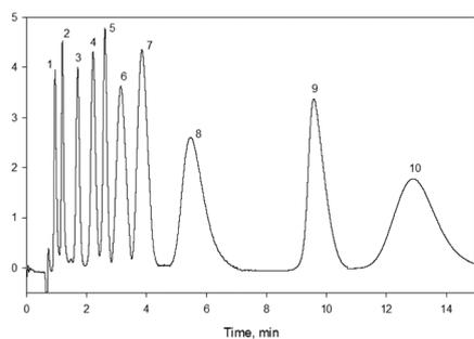
Fig. 7 Separation of 10 compounds using UiO-66(1x)@SiO<sub>2</sub>(5) column. Mobile phase – 20% ACN – 80% water, flow rate – 0.2 mL min<sup>-1</sup>, 25 °C, UV detection at 254 nm, 2 μL injections of 100 μg mL<sup>-1</sup> of analytes in mobile phase. Analytes numbered as in Table 3.
