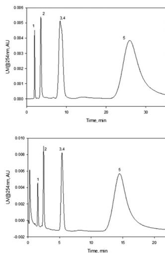
**Fig. 5** Separation of a mixture of PAH with 50 mm  $\times$  2.1 mm ID UiO-66@SiO<sub>2</sub> columns. Mobile phase – 0.2 ml min<sup>-1</sup> of *n*-hexane, 25 °C, 2  $\mu$ L injections of analytes (50  $\mu$ g mL<sup>-1</sup>) in mobile phase, UV detection at 254 nm. Analytes: 1 – benzene, 2 – anthracene, 3 – phenanthrene, 4 – naphthalene, 5 – pyrene. Columns: UiO-66(2x)@SiO<sub>2</sub>(5) (top) and UiO-66(1x)@SiO<sub>2</sub>(5) (bottom).
