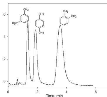
**Fig. 6** Separation of the mixture of xylene isomers using UiO-66(1x)@SiO<sub>2</sub>(5) column. Mobile phase – 40% ACN – 60% water, flow rate – 0.2 mL min<sup>-1</sup>, 25 °C, UV detection at 254 nm, 2  $\mu$ L injections of 50  $\mu$ g mL<sup>-1</sup> of analytes in mobile phase.
