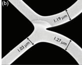
Fig. 2 Scanning electron micrographs (SEMs) of (a) the soft-glass single-ring ARR HC-PCF and (b) a close-up of a portion of the surrounding glass membranes. The fibre has a core diameter of  $\sim$ 25  $\mu$ m, and an average core wall thickness of 1.2 µm. The design reduces confinement loss by anti-resonant reflection between the core mode and modes of the surrounding single-ring.<sup>8</sup>
