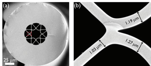
**Fig. 2** Scanning electron micrographs (SEMs) of (a) the soft-glass single-ring ARR HC-PCF and (b) a close-up of a portion of the surrounding glass membranes. The fibre has a core diameter of  $\sim 25$   $\mu\text{m}$ , and an average core wall thickness of 1.2  $\mu\text{m}$ . The design reduces confinement loss by anti-resonant reflection between the core mode and modes of the surrounding single-ring.<sup>8</sup>
