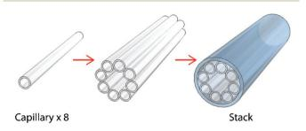
Fig. 1 Schematic illustration of the stacking procedure used to form the single-ring HC-PCF structure. More details on the "stack-and-draw" technique can be found in previous publications.4
