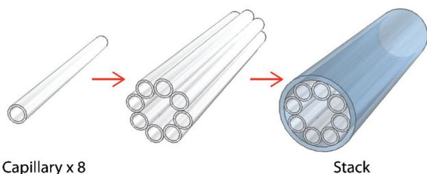
**Fig. 1** Schematic illustration of the stacking procedure used to form the single-ring HC-PCF structure. More details on the “stack-and-draw” technique can be found in previous publications.<sup>4</sup>
