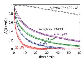
Fig. 5 (Symbols) Measured absorbance decay of a sample with an initial concentration  $C = 10 \mu M$  of  $(HBPz'_3)Rh(CO)_2$  in toluene, in a 35 cm-long soft-glass single-ring ARR HC-PCF. The colors correspond to different input powers. The grey data points correspond to a reference measurement in a 1 cm-long cuvette with  $C = 100 \mu M$ . The solid curves correspond to a mathematical model of the system (the values obtained for the quantum yield are summarized in Table 1).
