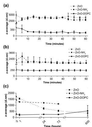
Fig. 5 DLS analysis comparing the behaviour of pristine ZnO NCs (dotted curve) and ZnO-DOPC NCs (solid curve) in terms of mean hydrodynamic size (z-average) in (a) SBF and (b) EMEM for both short (1 hour) and (c) long (25 days) time periods.
