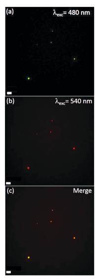
Fig. 3 Wide-field fluorescence image of the (a) lipid shell labeled by 1% Bodipy-DHPE; (b) ZnO-NH2 NCs conjugated with Atto550-NHS ester; and (c) the merged channels showing complete co-localization. Scale bar: 10 μm.
