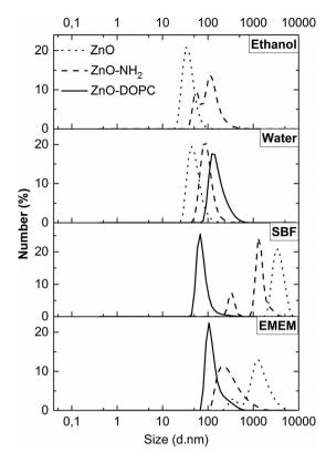
Fig. 4 Dynamic Light Scattering (DLS) measurements in number % of the ZnO samples, pristine ZnO NCs (dotted curves), ZnO-NH2 NCs (dashed curves), and ZnO-DOPC NCs (solid curves) in different media (ethanol, water, SBF, and EMEM).
