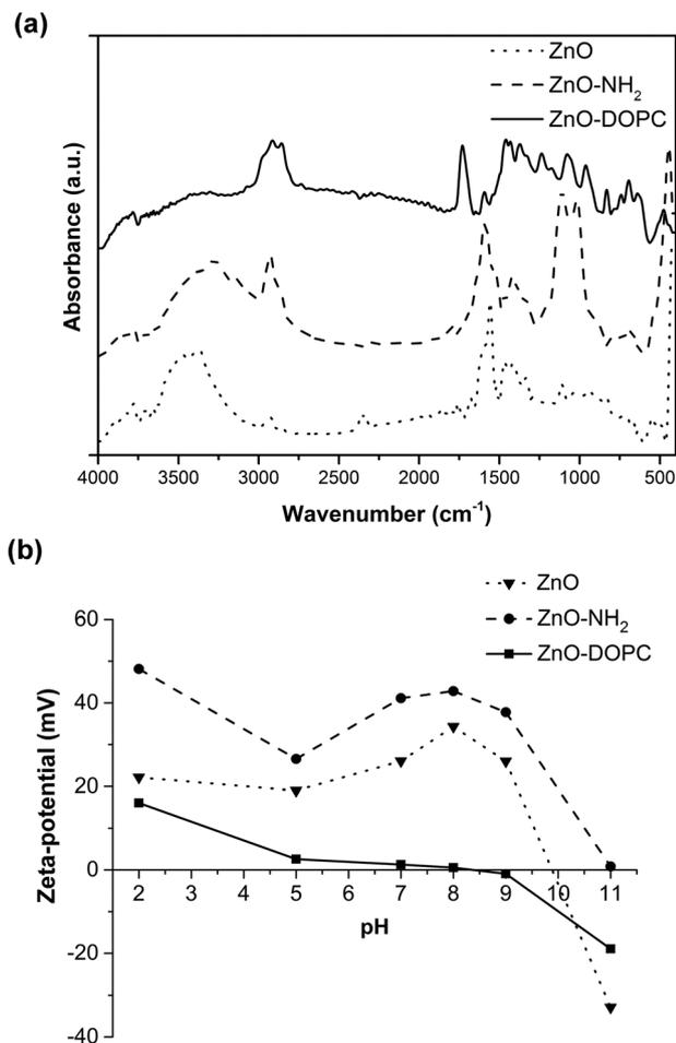
Fig. 2 (a) Fourier Transform-Infrared (FT-IR) spectra and (b) Z-potential measurements of the pristine ZnO and functionalized ZnO-NH<sub>2</sub> and ZnO-DOPC NCs.
