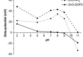
Fig. 2 (a) Fourier Transform-InfraRed (FT-IR) spectra and (b) Z-potential measurements of the pristine ZnO and functionalized ZnO-NH2 and ZnO-DOPC NCs.
