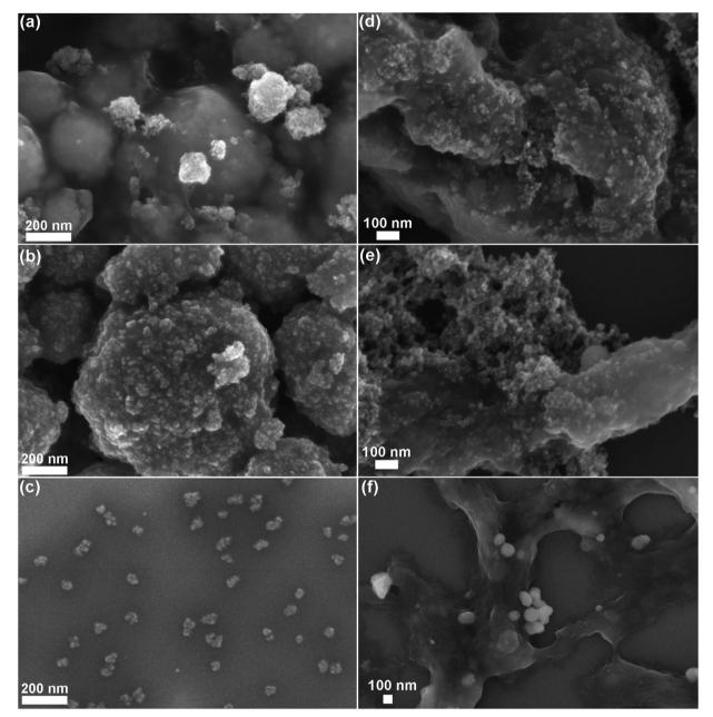
Fig. 6 FESEM images of the biostability behaviour of the three ZnO nanocrystals after 25 days assay times in SBF (left column) and EMEM (right column): (a–d) pristine ZnO, (b–e) ZnO–NH<sub>2</sub>, and (c–f) lipid-shell coated ZnO–DOPC.
