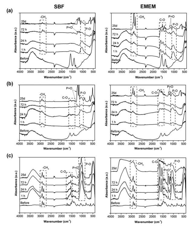
Fig. 7 Fourier-Transform InfraRed (FT-IR) spectra of the (a) pristine ZnO NCs, (b) ZnO-NH<sub>2</sub> NCs, and (c) ZnO-DOPC NCs after different time steps of biostability assays in SBF (left) and EMEM (right).
