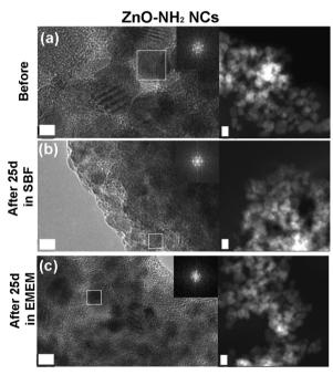
Fig. 9 HR-TEM, SAED and STEM imaging of the amine-functionalized ZnO-NH<sub>2</sub> nanocrystals: (a) before biostability treatments and in comparison after (b) 25 days in SBF solution and (c) 25 days in EMEM. The scale bar is 5 nm.
