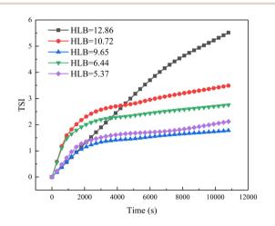
Fig. 5 TSI curves of emulsion under different emulsification system's HLB value ( $T=50~{\rm ^{\circ}C}$ ).
