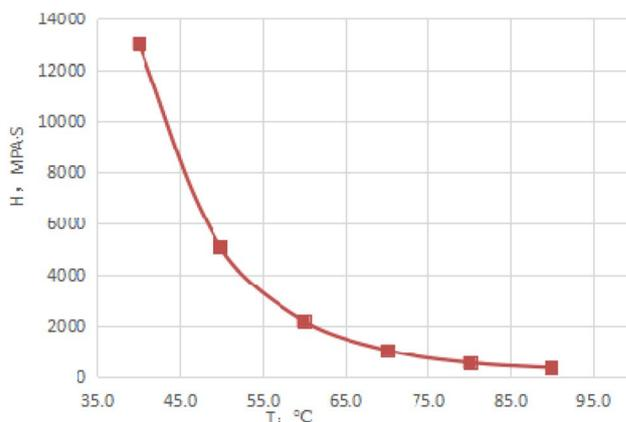
Fig. 2 Crude oil viscosity under different temperature.
