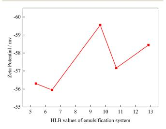
Fig. 8 Zeta potential of emulsion as a function of emulsification system's HLB value ( $T=50~{\rm ^{\circ}C}$ ).
