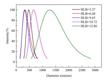
Fig. 7 Droplet size distributions of emulsion as a function of emulsification system's HLB value (T = 50 °C).
