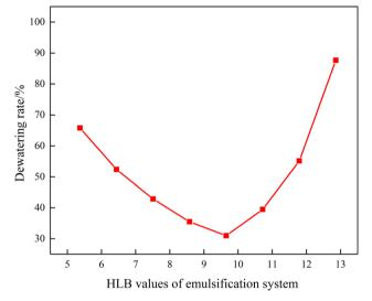
Fig. 4 Dewatering rate of emulsion with the variation of HLV values of compound system after 90 min (T=50 °C).
