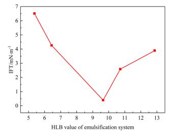
Fig. 9 Interfacial tension of emulsion as a function of emulsification system's HLB value ( $T=50~{\rm ^{\circ}C}$ ).
