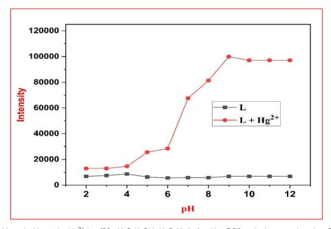
Fig. 12 pH effects with and without the  $Hg^{2+}$  ion [50  $\mu$ M  $C_2H_5OH-H_2O$  (4:1,v/v, pH=7.2)] excitation wave length = 500 nm and emission maxima wavelength of 584 nm at 25 °C.
