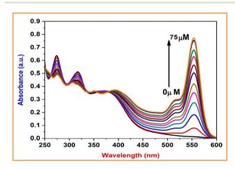
Fig. 3 UV-Vis spectral changes of L (40  $\mu$ M) upon steady addition of Hg<sup>2+</sup> ions in a HEPES buffer [50  $\mu$ M, C<sub>2</sub>H<sub>5</sub>OH-H<sub>2</sub>O (4:1, v/v, pH = 7.2)].
