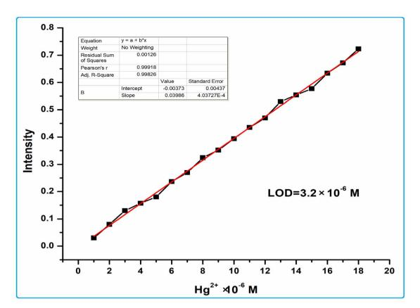
Fig. 6 Detection limit for  $Hg^{2+}$  from absorption titration in  $C_2H_5OH-H_2O$  (4:1, v/v).
