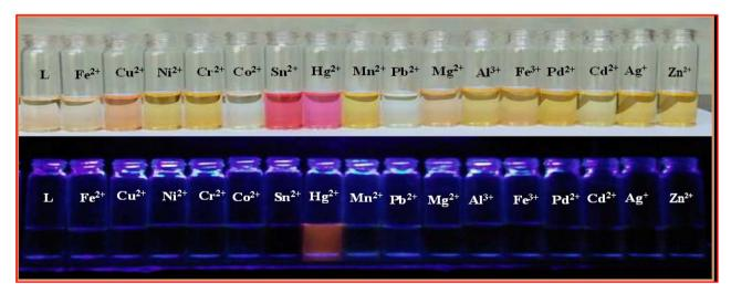
Fig. 2 Illustration of L and L + various metal ions: naked eye (upper part), under UV cabinet (lower part).
