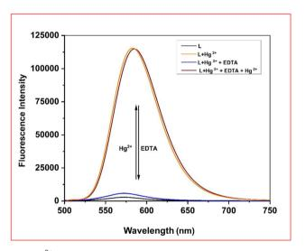
Fig. 9  $\,$  Hg<sup>2+</sup> complex of L (40  $\mu$ M) emission spectrum changes when EDTA is added in a HEPES buffer solution [50  $\mu$ M, C<sub>2</sub>H<sub>5</sub>OH-H<sub>2</sub>O (4:1, v/v, pH = 7.2)] at 25 °C. EDTA = 0-10 eq.
