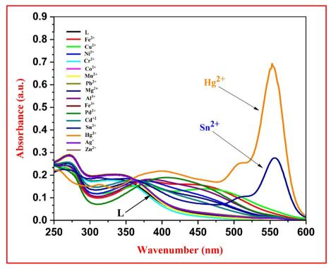
Fig. 1 UV-Vis spectra of L (40 μM) upon addition of various metal ions (Fe<sup>2+</sup>, Cu<sup>2+</sup>, Ni<sup>2+</sup>, Cr<sup>2+</sup>, Co<sup>2+</sup>, Sn<sup>2+</sup>, Hg<sup>2+</sup>, Mn<sup>2+</sup>, Pb<sup>2+</sup>, Mg<sup>2+</sup>, Al<sup>3+</sup>, Fe<sup>3+</sup>, Pd<sup>2+</sup>, Cd<sup>2+</sup>, Ag<sup>+</sup> and Zn<sup>2+</sup>) in a HEPES buffer [C<sub>2</sub>H<sub>5</sub>OH-H<sub>2</sub>O (4:1,v/v) pH = 7.2] at 25 °C.
