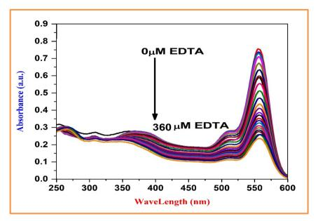
Fig. 4 UV-Vis spectral changes of  $Ha^{2+}$  complex of L upon addition of EDTA in  $C_2H_5OH-H_2O$  (4:1, v/v).
