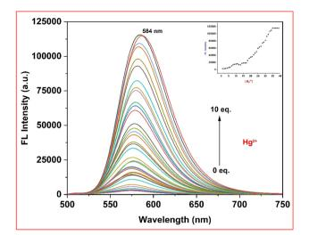
Fig. 8 (a) Changes in the emission spectrum of L (40  $\mu$ M) at 25 °C after the addition of the Hg<sup>2+</sup> ion in a HEPES buffer [50  $\mu$ M, C<sub>2</sub>H<sub>5</sub>OH–H<sub>2</sub>O (4 : 1, v/v, pH = 7.2)] [Hg<sup>2+</sup>] = 0–10 eq. (b) Inset: 584 nm intensity vs. the quantity of equivalent Hg<sup>2+</sup> added.
