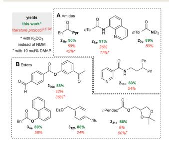
Scheme 6 Comparison of the present method with the literature method<sup>15a</sup> employing TCT and NMM. <sup>a</sup>For reaction conditions see Schemes 3 and 5; yields refer to the isolated material after chromatographic purification or distillation. <sup>b</sup>For reaction conditions see Scheme 1A and Chapter 4, ESI;† yield determined with an internal NMR standard.
