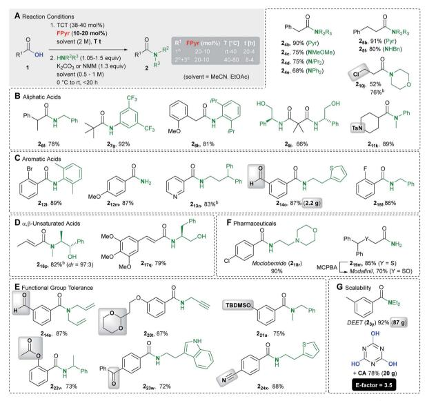
Scheme 3 Synthesis of amides of type 2. <sup>a</sup>lsolated yield after chromatography or distillation if not mentioned otherwise. <sup>b</sup>Yield determined by means of an internal NMR standard. <sup>c</sup>With 1.3 equiv. 1, 49 mol% TCT, 1.7 equiv. NMM and 1.0 equiv. nucleophile. Pyr = N-pyrrolidyl, Ts = para-tolylsulfonyl, and TBDMS = tert-butyldimethylsilyl.
