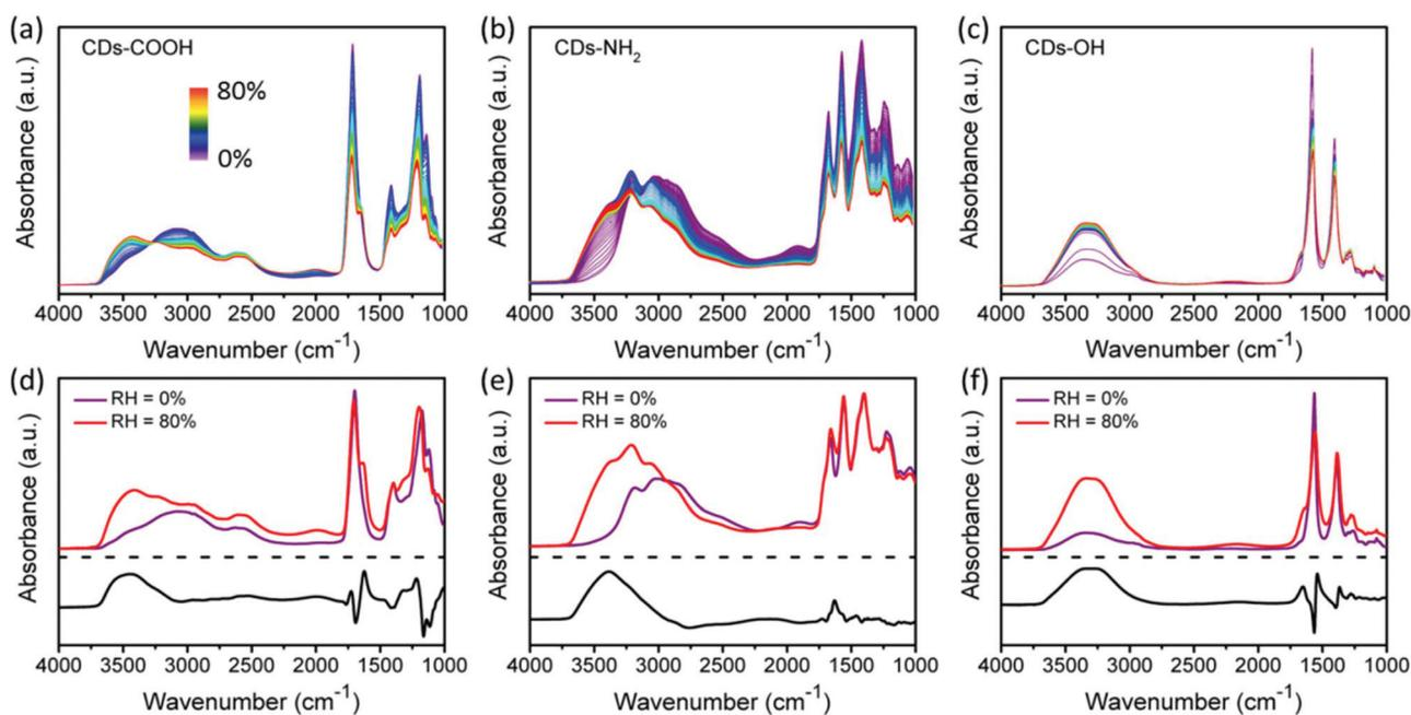
Fig. 5 (a)–(c) FTIR spectra of carbon dot samples recorded at different relative humidity values; (d)–(f) normalized FTIR spectrum obtained from the dry state and that from a humid atmosphere; the lower panel shows the difference spectrum.
