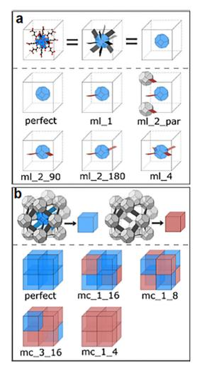
**Fig. 8** Depiction of (a) missing-linker defects (ml is referred to missing linker, followed by the number and, where applicable, the relative positions where linkers were detached) and (b) missing-cluster defects and relating supercells (mc\_1\_4, mc\_3\_16, mc\_1\_8, and mc\_1\_16 (mc = missing cluster) stand for defects with 1/4, 3/16, 1/8, and 1/16 of the total number of clusters removed). Reprinted with permission from ref. 247 Copyright 2019 American Chemical Society.
