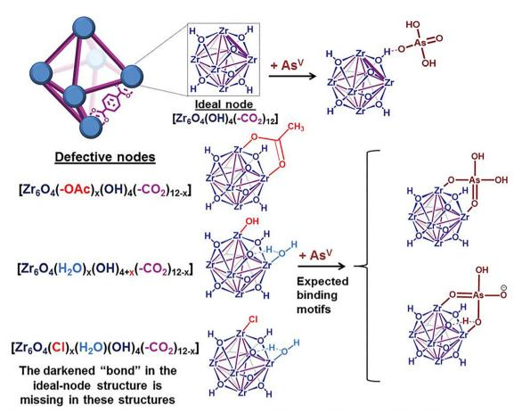
Fig. 11 Structural scheme of ideal and missing-linker defective UiO-66, with either 12-coordinated ideal [Zr<sub>6</sub>O<sub>4</sub>(OH)<sub>4</sub>(-CO<sub>2</sub>)<sub>12</sub>] or defective [Zr<sub>6</sub>O<sub>4</sub>(OH)<sub>X</sub>(-CO<sub>2</sub>)<sub>v</sub>] nodes. Reprinted with permission from ref. 282 Copyright 2016 Royal Society of Chemistry.
