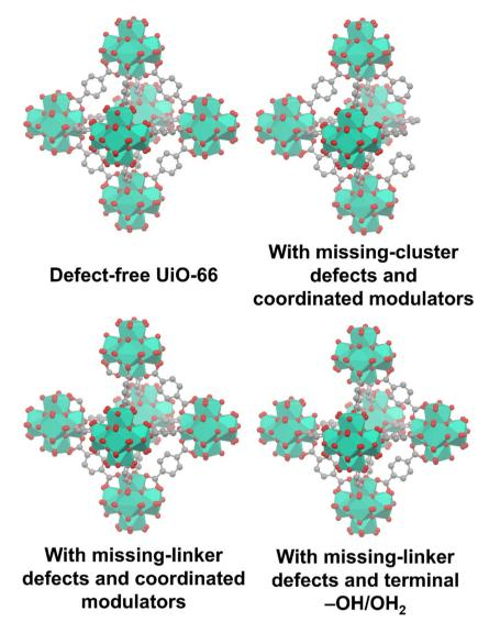
Common defects in a zirconium-based MOF, UiO-66. Hydrogen atoms are not shown in all structures.
