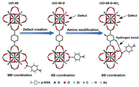
Fig. 5 Synergistic mechanism of UiO-66-D-NH<sub>2</sub> for adsorption of organoarsenic (MM = monodentate mononuclear As-Zr complex, BB = bidentate binuclear As-Zr complex). Reprinted from ref. 238 Copyright 2019 Royal Society of Chemistry.
