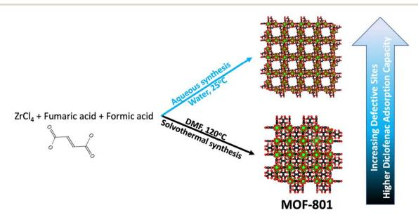
Fig. 4 Schematic synthesis of defective MOF-801 for DCF adsorption. Reprinted from ref. 236 Copyright 2022 Elsevier.
