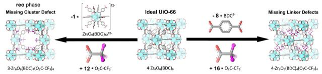
Fig. 12 Structural scheme and compositional differences between the ideal and defective UiO-66 samples. Reprinted with permission from ref. 34 Copyright 2016 American Chemical Society
