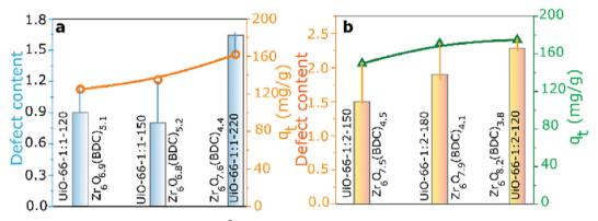
Fig. 17 The relationship between the defect density and Pb<sup>2+</sup> removal (a) and (b). Reprinted with permission from ref. 178 Copyright 2021 American Chemical Society.
