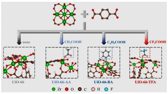
Synthetic design of the UiO-66-X with different modulators. Reprinted with permission from ref. 293 Copyright 2022 Elsevier.
