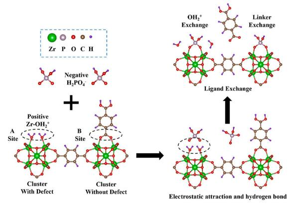
Fig. 9 Phosphate adsorption on nodes of linker-defective UiO-66. Binding at site A entails displacement of node agua and terminal-hydroxo ligands (rather than pairs of aqua ligands, as sketched). At site B, phosphate binds via displacement of carboxylate-terminated linkers. Reprinted with permission from ref. 280 Copyright 2021 Elsevier
