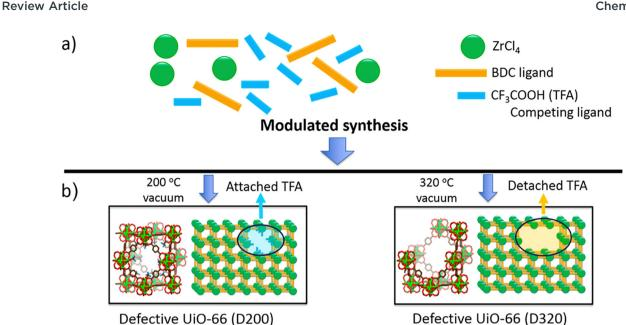
Fig. 7 (a) Illustration of defective UiO-66 with TFA and (b) proposed structural conversions after post-synthetic heat reaction. Reprinted with permission from ref. 241 Copyright 2017 American Chemical Society.
