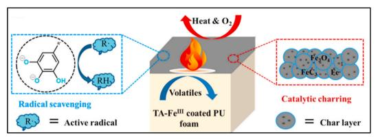
Fig. 1 Mechanism scheme of TA-Fe<sup>III</sup> MPN flame retardant. Reproduced with permission from ref. 65. Copyright (2021) Elsevier.
