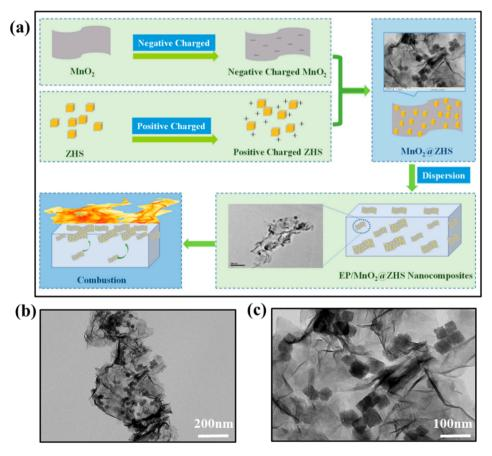
Fig. 13 (a) Synthesis of MnO<sub>2</sub>@ZHS hybrids and flame retardancy mechanism in epoxy; (b and c) TEM images of MnO<sub>2</sub>@ZHS hybrids. Reproduced with permission from ref. 115. Copyright (2019) Polymers.
