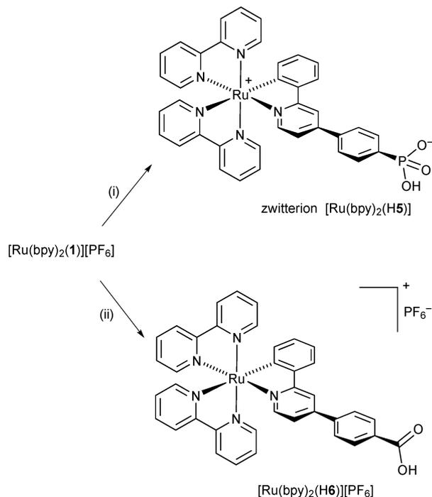
**Scheme 5** Conversion of  $[\text{Ru}(\text{bpy})_2(\mathbf{1})][\text{PF}_6]$  to  $[\text{Ru}(\text{bpy})_2(\text{H5})]$  and  $[\text{Ru}(\text{bpy})_2(\text{H6})][\text{PF}_6]$ . Optimized conditions: (i)  $\text{H}_2\mathbf{4}$ ,  $\text{K}_3\text{PO}_4$ , SPhos Pd G2, MeCN/ $\text{H}_2\text{O}$ ; 70 °C, 5 h; (ii) 4-carboxyphenylboronic acid,  $\text{K}_3\text{PO}_4$ , SPhos Pd G2, MeCN/ $\text{H}_2\text{O}$ ; 70 °C, 5 h.
