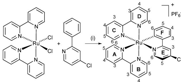
**Scheme 3** Cyclometallation reaction to form [Ru(bpy)<sub>2</sub>(1)][PF<sub>6</sub>]. Conditions: (i) AgPF<sub>6</sub>, CH<sub>2</sub>Cl<sub>2</sub>, reflux, 19 h. Ring and atom labels used for NMR assignments are shown.
