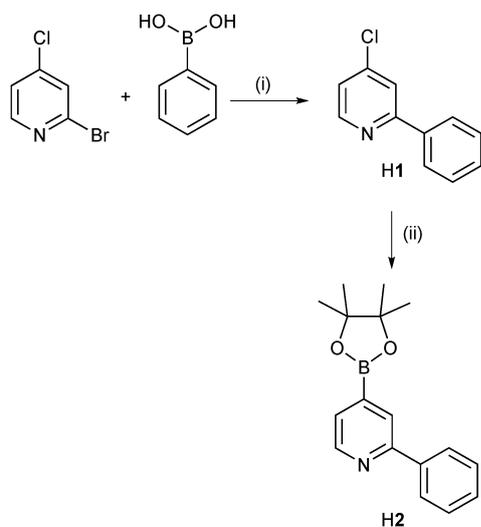
**Scheme 2** Syntheses of intermediates H1 and H2. Conditions: (i) Na<sub>2</sub>CO<sub>3</sub>, [Pd(PPh<sub>3</sub>)<sub>2</sub>Cl<sub>2</sub>], THF/H<sub>2</sub>O, 60 °C, 3 h; (ii) bis(pinacolato)diboron, KOAc, [Pd(dppf)Cl<sub>2</sub>], dioxane, reflux, 72 h.
