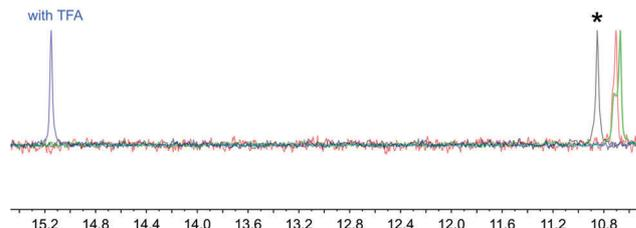
**Fig. 5** 162 MHz  $^{31}\text{P}\{^1\text{H}\}$  NMR spectrum of  $[\text{Ru}(\text{bpy})_2(\text{H5})]$  (\*) in  $\text{CD}_3\text{OD}$ , and spectra taken after the addition of (a)  $\text{CF}_3\text{CO}_2\text{H}$  (TFA, blue), (b)  $\text{K}_2\text{CO}_3$  (green) or (c)  $\text{CF}_3\text{CO}_2\text{H}$  followed by  $\text{K}_2\text{CO}_3$  (red).
