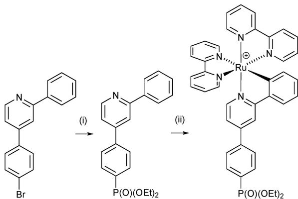
Scheme 1 Previously reported synthesis<sup>16</sup> of a phosphonate ester-functionalized  $[\text{Ru}(\text{N}^{\wedge}\text{N})_2(\text{C}^{\wedge}\text{N})]^+$  complex. Conditions: (i)  $[\text{Pd}(\text{PPh}_3)_4]$ ,  $\text{Cs}_2\text{CO}_3$ ,  $\text{HPO}(\text{OEt})_2$ , THF, microwave, 110 °C, 90 min; (ii) *cis*- $[\text{Ru}(\text{bpy})_2\text{Cl}_2]$ ,  $\text{AgPF}_6$ .
