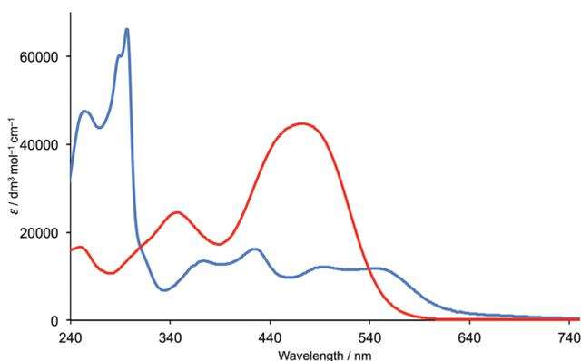
Fig. 6 The solution absorption spectra of  $[\text{Ru}(\text{bpy})_2(\text{H5})]$  (MeOH,  $1 \times 10^{-5}$  mol  $\text{dm}^{-3}$ , blue curve) and of the dye P1 (MeCN,  $1 \times 10^{-5}$  mol  $\text{dm}^{-3}$ , red curve).
