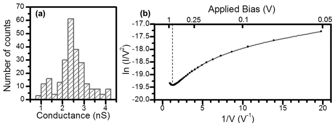
Fig. 10 (a) Conductance histogram built from all the experimental data from  $-0.5$  to  $0.5$  V for each  $I$ - $V$  curve recorded (ca. 250 curves) positioning the tip onto an AgNP and applying a set point force of  $17.5$  nN. (b) The solid squares represent the average of 10  $I$ - $V$  curves for a **1AgNP** device. The dashed vertical line corresponds to the voltage at which the tunnelling barrier transition occurs ( $V_{\text{trans}}$ ).
