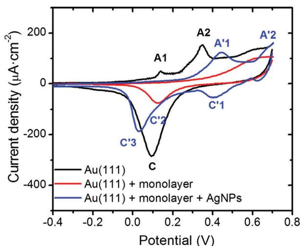
Fig. 11 Black: cyclic voltammograms recorded for a bare Au(111) electrode. Red: monolayer of **1H<sub>2</sub>** transferred onto a Au(111) substrate. Blue: Au(111)/monolayer with overlying silver nanoparticles (**1AgNP**). All the voltammograms were recorded in a  $0.1$  M NaOH aqueous solution at  $0.1$  V  $s^{-1}$  using a Ag/AgCl, KCl ( $3$  M) reference electrode.
