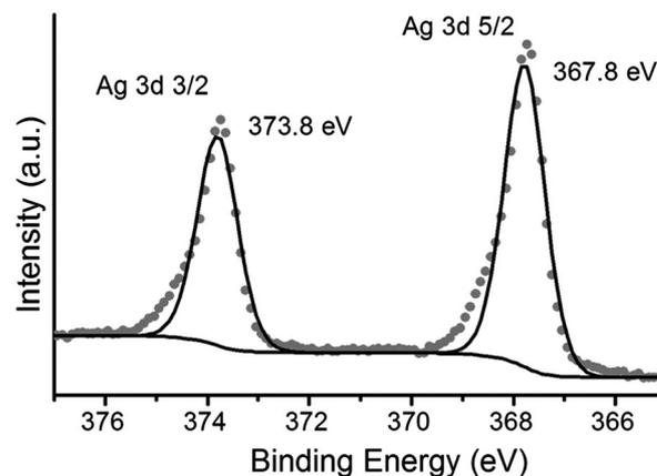
Fig. 5 XPS spectrum of Ag(3d) photoelectrons of a one-layer LB film of  $1\text{AgNP}$ , formed following transference of a LB film of  $1\text{Ag}^+$  from an  $\text{AgNO}_3$  aqueous solution and irradiated at 254 nm for 15 minutes.
