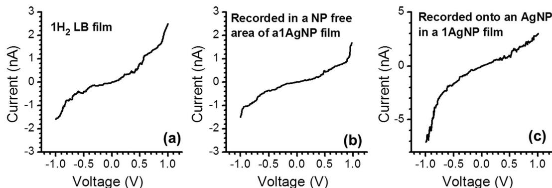
**Fig. 9** Representative  $I$ - $V$  curves for the indicated films. The set-point force used was 8 nN for (a) and (b) and 17.5 nN for (c).
