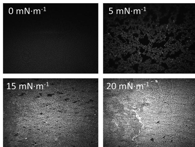
Fig. 3 Brewster Angle Microscopy images of Langmuir films formed from **1H<sub>2</sub>** on an  $\text{AgNO}_3$  aqueous sub-phase (**1HAg<sup>+</sup>**) at the indicated surface pressures. The collapse of the monolayer can be observed in the bottom right image. The field of view along the x axes for the BAM images is 3300  $\mu\text{m}$ .
