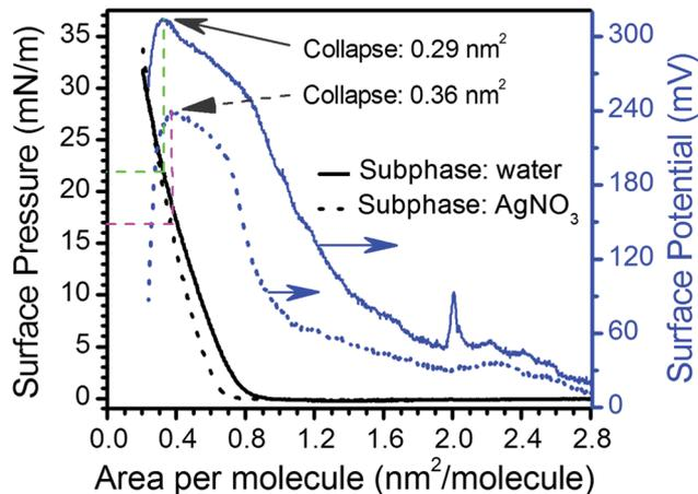
Fig. 2 Representative surface pressure and surface potential *vs.* area per molecule isotherms formed from **1H<sub>2</sub>** on pure water (**1H<sub>2</sub>**) and  $4 \times 10^{-4}$  M  $\text{AgNO}_3$  (**1HAg<sup>+</sup>**) aqueous sub-phases.
