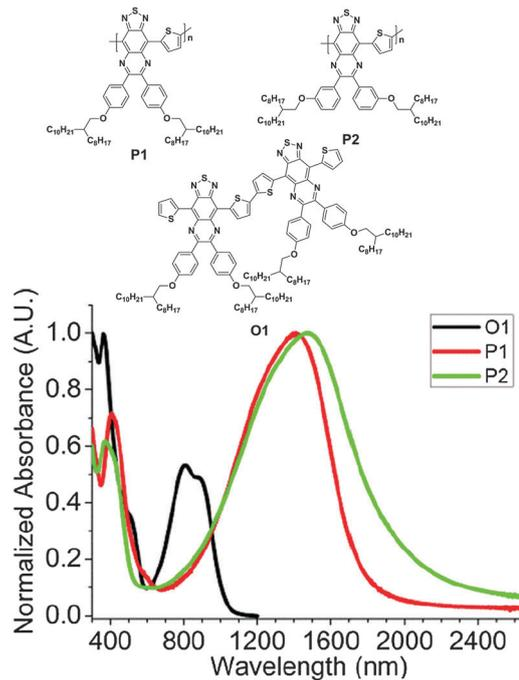
Fig. 6 Chemical structures and UV-vis-NIR absorption spectra of thin films of O1, P1, and P2. Reprinted with permission from the publisher.<sup>62</sup>
