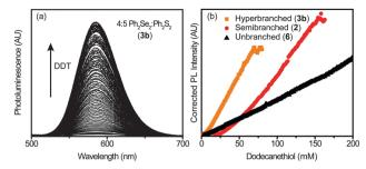
Fig. 5 (a) Steady-state PL of 3b in the presence of dodecanethiol (DDT). Increasing the amount of thiol leads to a concomitant increase in Mn<sup>2+</sup> PL from the NCs. (b) Scatter plot of the Mn<sup>2+</sup> PL intensity vs. [DDT] for NC samples with different degrees of branching. The more branched 3b NCs show the steepest increase in PL intensity with thiol. NCs with less (2) and no (6) branching show decreasing sensitivity to thiol, with smaller increases in slope.
