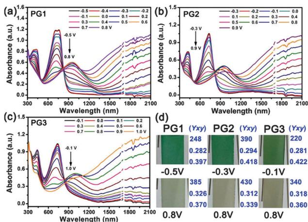
Fig. 3 Spectroelectrochemistry of PG1, PG2 and PG3 film on an ITO-coated glass slide (0.5 cm width) in a monomer-free 0.1 M TBAPF<sub>6</sub>/ACN electrolyte–solvent couple at applied potentials: (a) –0.5 to 0.8 V, (b) –0.3 to 0.9 V, (c) –0.1 to 1.0 V. (d) Photographs and corresponding (Y; x; y) values of PG1, PG2 and PG3 film on an ITO-coated glass slide in the fully neutral and oxidized states.
