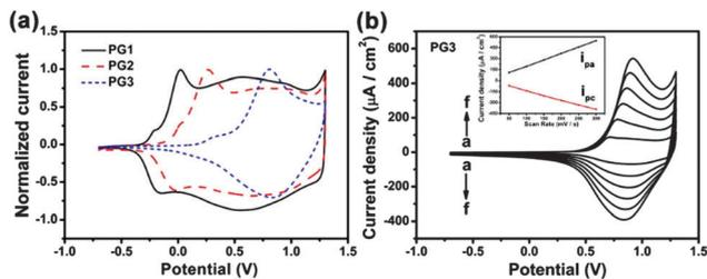
Fig. 2 (a) Single scan cyclic voltammograms of different films at 100 mV s<sup>-1</sup> in 0.1 M TBAPF<sub>6</sub>/ACN: PG1 (black, solid line), PG2 (red, dashed line), and PG3 (blue, short dashed line). (b) Scan rate dependence of the PG3 film in 0.1 M TBAPF<sub>6</sub>/ACN at (a) 50, (b) 100, (c) 150, (d) 200, (e) 250 and (f) 300 mV s<sup>-1</sup> (inset is the plot of scan rate with anodic (*i*<sub>pa</sub>) and cathodic (*i*<sub>pc</sub>) peak currents).
