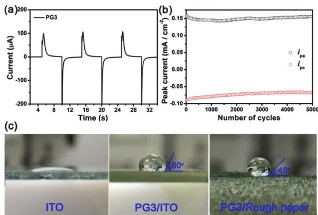
Fig. 4 (a) Chronoamperometry for PG3 with a 5 s delay for each potential ( $-0.1$  V and  $+0.8$  V). (b) Stability of a 600 nm thick PG3 film cycled 5000 times with a scan rate of  $100$   $\text{mV s}^{-1}$  in  $0.1$  M TBAPF<sub>6</sub>/ACN: the change in the anodic ( $\square$ ) and cathodic ( $\circ$ ) peak currents as a function of number of cycles. (c) Photographs of the water droplet volume of  $10$   $\mu\text{L}$  on the surface of ITO, PG3/ITO and PG3/rough paper, respectively.
