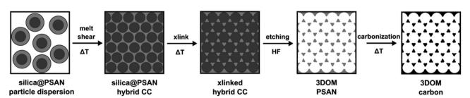
Fig. 2 Overview scheme for the fabrication of 3D-ordered porous carbonaceous materials within this study
