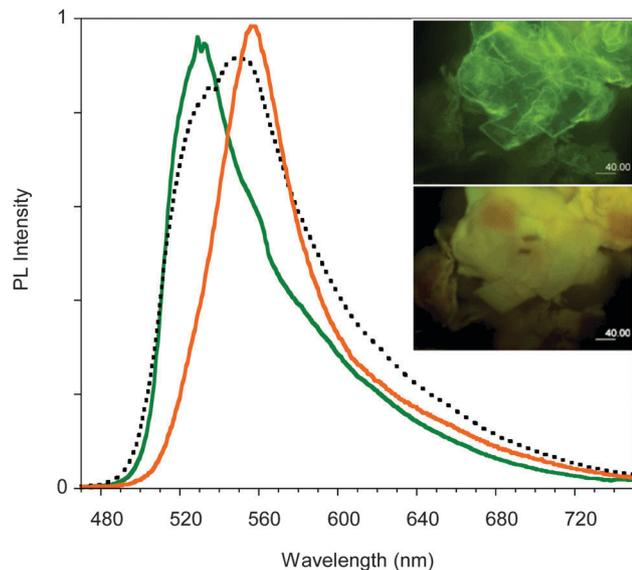
Fig. 11 PL spectra of crystals of **D** before thermal treatment (green line), after treatment at 50 °C for 10 min (dotted black line) and 25 min (orange line). Inset: Images taken at the microscope before (top) and after (bottom) thermal treatment.
