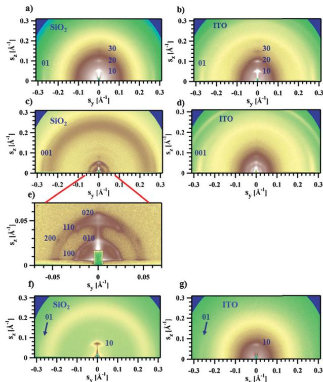
Fig. 5 GIWAXS patterns for OFET (left) or SCLC (right) devices for  $P_a$  [(a) and (b)],  $T_a$  [(c) and (d)] and  $T_b$  [(f) and (g)]. (e) is an enlarged small-angle region of image in (c). The incidence angle is  $0.2^\circ$ .
