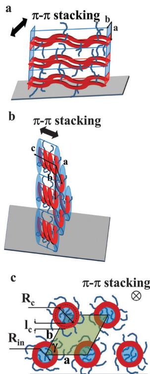
Fig. 6 Models schematically depicting the layer-like structure of thin films of  $\mathbf{P}_a$  (a) and  $\mathbf{T}_a$  (b). The polymer backbone is represented in red while the film surface is the gray parallelogram. (c) The view along the helical axis represents notations used in eqn (7) and (8). The inner part of the helices is colored in blue, the area of the pseudo-hexagonal unit cell external to the helices is colored in green (c).
