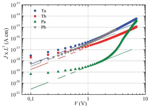
Fig. 2 Space-charge-limited current on as-cast polymers. For **P<sub>a</sub>** the curve has been obtained by averaging the current–voltage data of four devices processed under identical conditions. The dashed lines correspond to a fit in the voltage range where  $J$  follows a square-law dependence (constant mobility) on the voltage.
