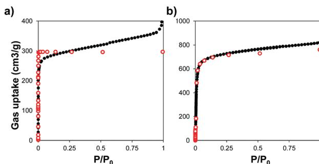
Fig. 2 N<sub>2</sub> adsorption isotherms measured at 77 K for (a) Zr–L1 and (b) Zr–L7. Experimental (black close dots) and GCMC simulated (red open dots) data.
