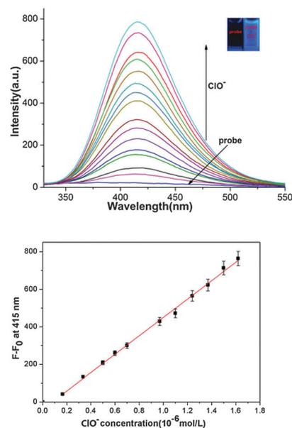
**Fig. 2** Top: Fluorescence spectra of **1** (2.5  $\mu\text{M}$ ) in the presence of various concentrations of  $\text{ClO}^-$  (0–1.8  $\mu\text{M}$ ) in HEPES (10 mM, pH 7.4) ( $\lambda_{\text{ex}} = 300$  nm). Bottom: Plot of intensities of fluorescence at 415 nm as a function of the concentrations of  $\text{ClO}^-$ .
