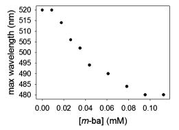
Fig. 5 (top) A blue shift in the absorbance spectrum of an aqueous solution of ARS is observed as PAMAM-m-ba is added. (bottom) The position of the absorption maximum at around 500 nm as a function of the added polymer. T = 25 °C; pH = 7.4 in 50 mM HEPES; [ARS] =  $5.208 \times 10^{-5}$  M.
