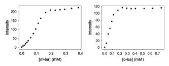
**Fig. 4** Binding titration of **ARS** dye with **PAMAM-***m***-ba** (left) and **PAMAM-***o***-ba** (right) monitored by fluorescence emission intensity. T = 25 °C; pH = 7.4 in 50 mM HEPES; [**ARS**] =  $5.257 \times 10^{-5}$  M;  $\lambda_{\text{exc}} = 518$  nm;  $\lambda_{\text{em}} = 545$  nm.
