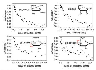
Fig. 8 Sugar binding monitored by the changes in fluorescence anisotropy associated with the displacement of ML dye from a [PAMAM-m-ba-ML] complex at pH 10 in water (50 mM CAPS). T = 25 °C; [ML] = 1.057  $\times$  $10^{-5}$  M; [**PAMAM-***m***-ba**] = 1.737 ×  $10^{-5}$  M;  $\lambda_{\rm exc}$  = 384 nm;  $\lambda_{\rm em}$  = 450 nm. Insets: chemical structures and names of the simple sugars studied.
