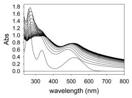
Fig. 6 Changes in the absorption of [PAMAM-m-ba·ARS] over the course of 47 min (spectra acquired every 2 min). T = 25 °C; pH = 7.4 in 50 mM HEPES; [ARS] =  $5.10 \times 10^{-5}$  M; [PAMAM-m-ba] =  $4.50 \times 10^{-5}$  M
