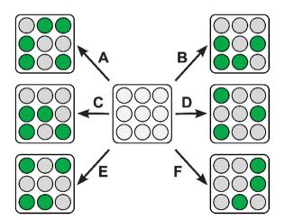
Scheme 5 A pattern-based sensing array. The array, composed of multiple receptors (centre) is exposed to each analyte in turn (A-F). Sensors in the array are not selective for any of the analytes, but the overall response of the whole array generates a unique and recognizable "finger print" of each analyte, which allows for selective recognition.
