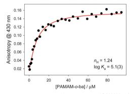
Fig. 2 Binding isotherm obtained from addition of **PAMAM-o-ba** to **ML**. The experimental data were fit to a modified Hill isotherm (red)  $r = (r_{\text{max}} - r_{\text{min}}) [\text{PAMAM-o-ba}]^n / ([\text{PAMAM-o-ba}]^n + (1/K_a)^n) + r_{\text{min}}. T = 25 °C; pH = 7.4 in water (50 mM HEPES); [ML] = <math>1.027 \times 10^{-5}$  M;  $\lambda_{\text{exc}} = 362$  nm;  $\lambda_{\text{em}} = 450$  nm.
