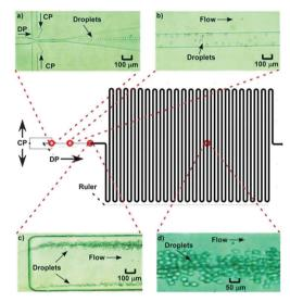
Fig. 6 Photographs of droplets (a) being generated at the flow focusing junction, (b) in the 10  $\mu m$  deep channel, (c) entering the 60  $\mu m$  deep serpentine channel, and (d) inside the serpentine channel where they would undergo UV polymerisation
