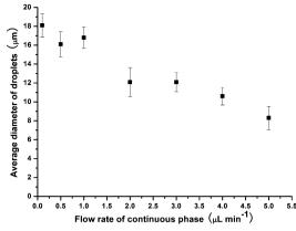
Fig. 5 Control of droplet size by varying the flow rate of the aqueous continuous phase, with the dispersed phase flow rate held constant at  $0.5 \mu L min^{-1}$
